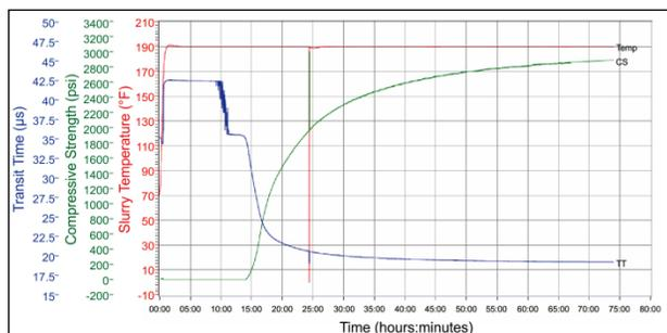
**Figure 4: Compressive strength development for the slurry Class G cement 15.8 lb/gal, CD-1 (0.5% bwoc), HMHAG (0.4% bwoc), D3 (1.0% bwoc)**
