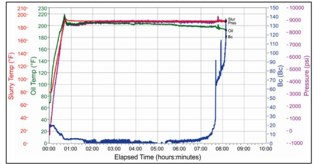
**Figure 2: Thickening time graph for the slurry: Class G cement 15.8 lb/gal, CD-1 0.5% bwoc, HMHAG 0.4% bwoc, EAD-D8 0.5 gal/sack**
