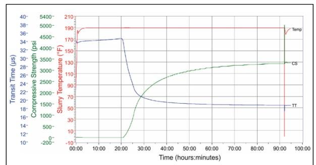
**Figure 3: Compressive strength development for the slurry Class G cement 15.8 lb/gal, CD-1 0.5% bwoc, HMHAG 0.4% bwoc, EAD-D8 (powder form) 1.77% bwoc**
