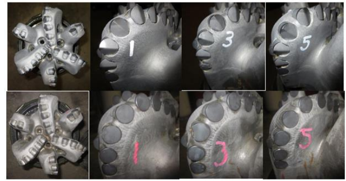
Fig. 16—RDE-equipped drill bit dull (top) and standard-cutter-equipped drill bit dull (below)
