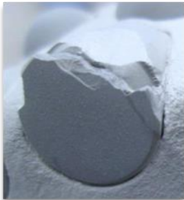
Fig. 2—Impact-damaged PDC cutter.
