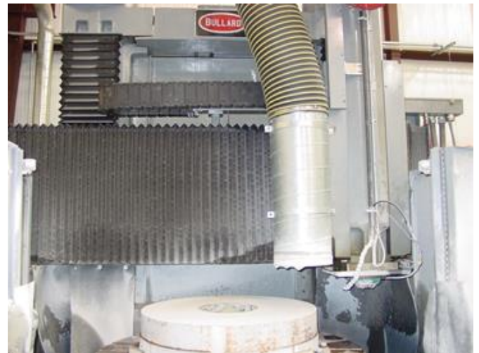
Fig. 7—A VTL with a granite log.
