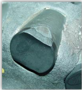
Fig. 1—Wear-damaged PDC cutter.
