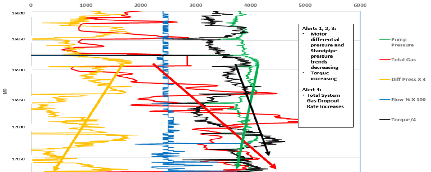
Figure 6: Horizontal Wellbore Collapse
