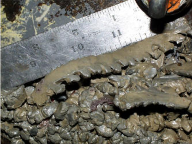
Figure 29. Cuttings from six blade 6½ inch PDC bit with WBM.
