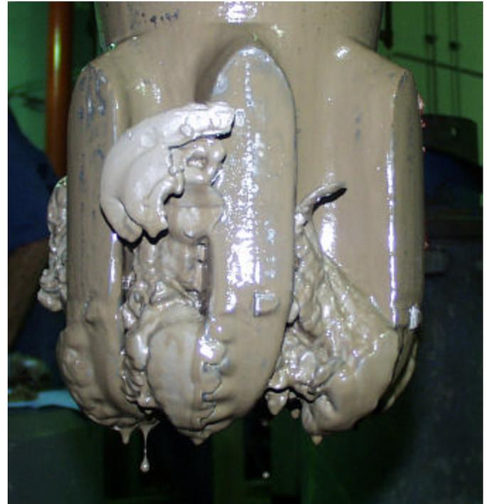
**Figure 18. Six blade 8½ inch PDC bit with non-polished cutters and WBM.**
