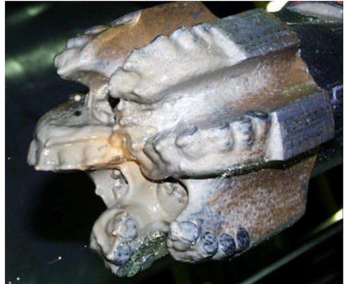
Figure 32. Six blade 6½ inch PDC bit with SBM.
