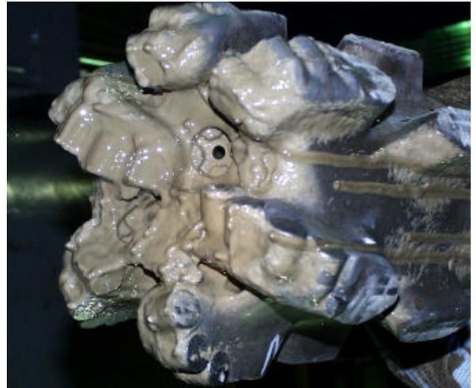
Figure 24. Six blade 7-7/8 inch PDC bit with worn cutters and SBM.
