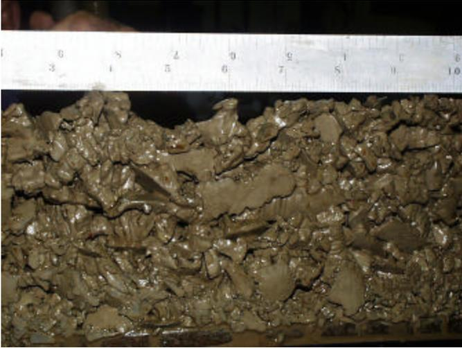
Figure 5. Cuttings from three blade 8½ inch PDC bit with WBM.
