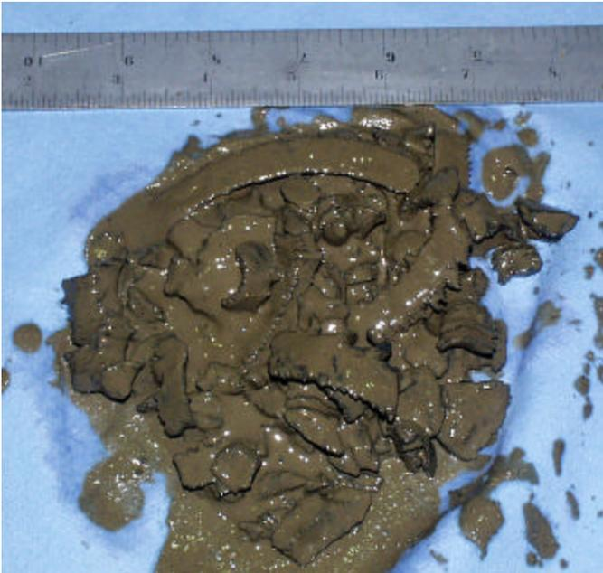
Figure 25. Cuttings from six blade 7-7/8 inch PDC bit with worn cutters and SBM.
