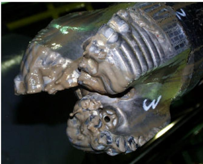
Figure 3. Three blade 8½ inch PDC bit with WBM + Drilling Enhancer.
