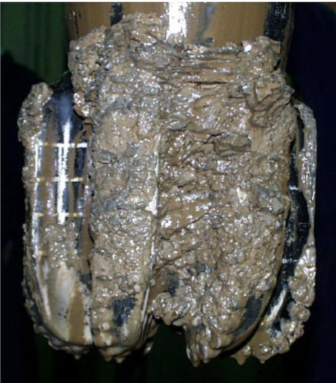
Figure 15. Six blade 8½ inch PDC bit rpm test with WBM.
