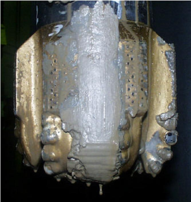
Figure 31. Six blade 6½ inch PDC bit with WBM + Drilling Enhancer.
