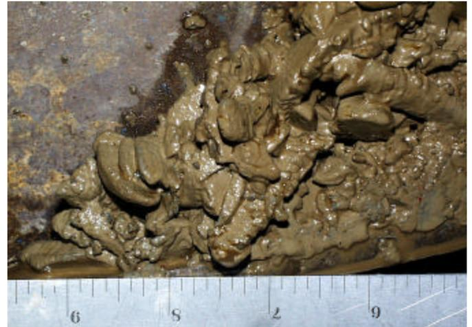
Figure 16. Cuttings from six blade 8½ inch PDC bit rpm test with WBM.
