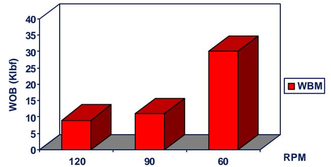
Figure 14: RPM Test - Six Blade PDC Bit
