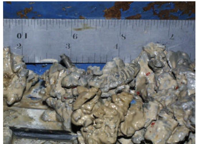
**Figure 20. Cuttings from six blade 8½ inch PDC bit with non-polished cutters and WBM + Drilling Enhancer.**
