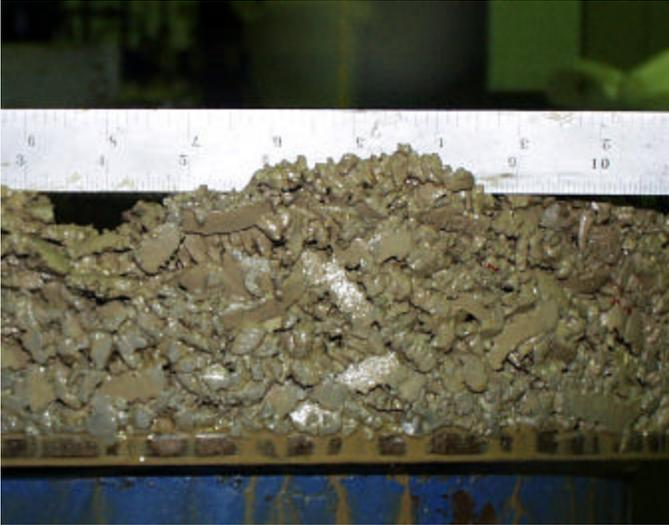
Figure 13. Cuttings from six blade 8½ inch PDC bit with WBM + Drilling Enhancer.
