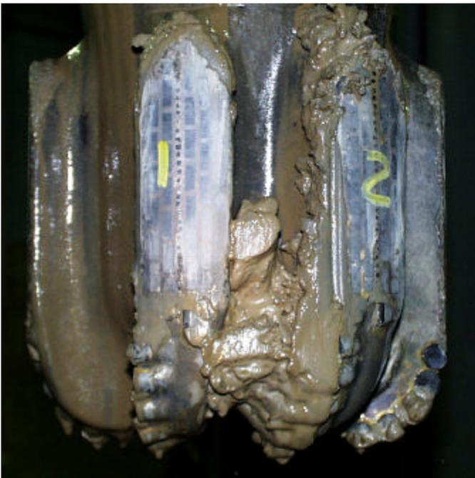
**Figure 19. Six blade 8½ inch PDC bit with non-polished cutters and WBM + Drilling Enhancer.**
