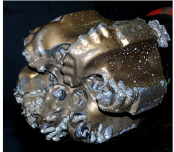
Figure 26. Six blade 6 1/2 inch PDC bit with WBM.
