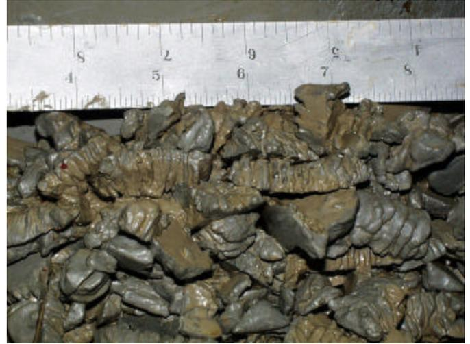
Figure 6. Cuttings from three blade 8½ inch PDC bit with WBM + Drilling Enhancer.
