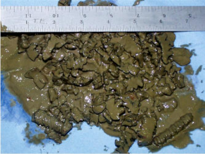
**Figure 33. Cuttings from six blade 6½ inch PDC bit with SBM.**
