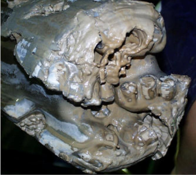
Figure 21. Six blade 7-7/8 inch PDC bit with worn cutters and WBM + Drilling Enhancer.
