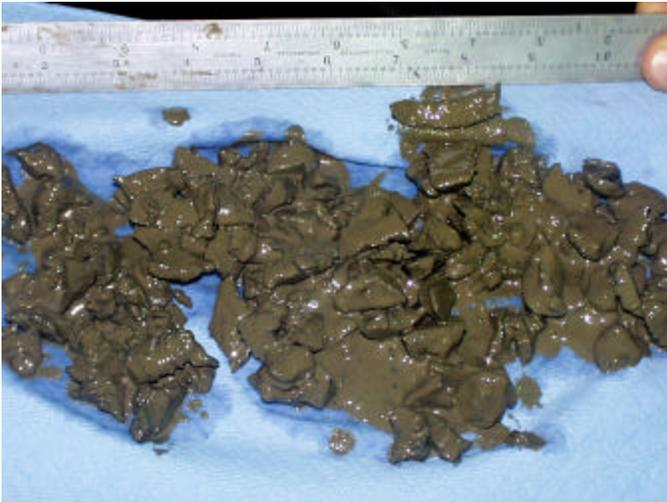
Figure 7. Cuttings from three blade 8½ inch PDC bit with SBM.
