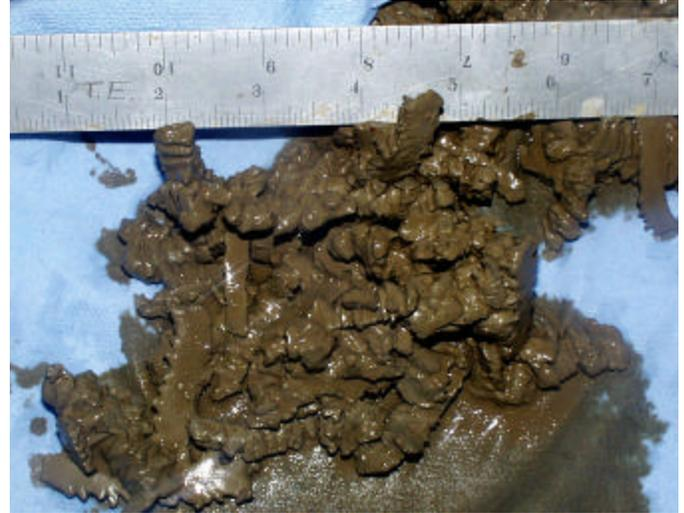
Figure 30. Cuttings from six blade 6½ inch PDC bit with WBM + Drilling Enhancer.
