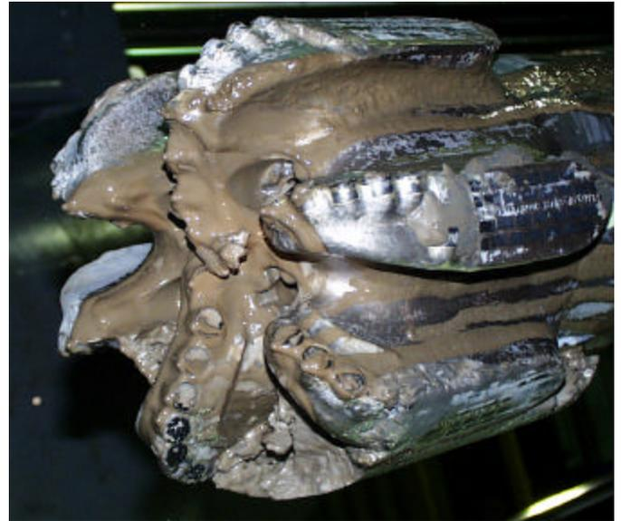
Figure 8. Six blade 8½ inch PDC bit with WBM + Drilling Enhancer.
