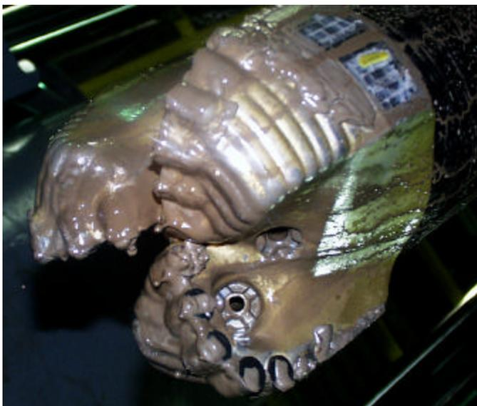
Figure 1. Three blade 8½ inch PDC bit with WBM.
