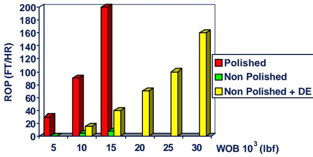
**Figure 17: Six Blade PDC Bit - Non-Polished Cutters**
