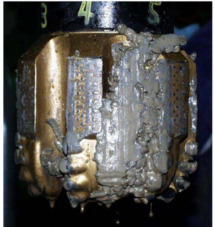
Figure 28. Six blade 6 1/2 inch PDC bit with WBM.
