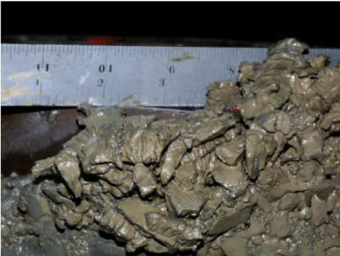
Figure 23. Cuttings from six blade 7-7/8 inch PDC bit with worn cutters and WBM + Drilling Enhancer.
