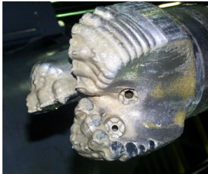
Figure 4. Three blade 8½ inch PDC bit with SBM.
