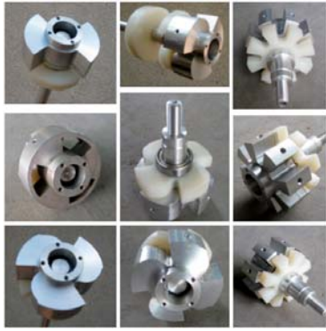
Fig. 5d - Some sirens tested in wind tunnel.
