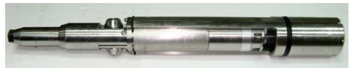
Fig. 1a - Prototype single-siren tool (assembled).
