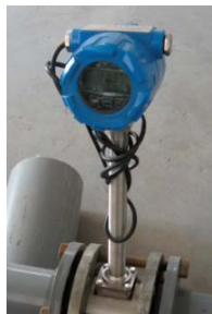
Fig. 5g - Flow meter.
