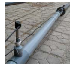
Fig. 5m - Piezoelectric transducer closest to siren for constructive interference and harmonic generation study.
