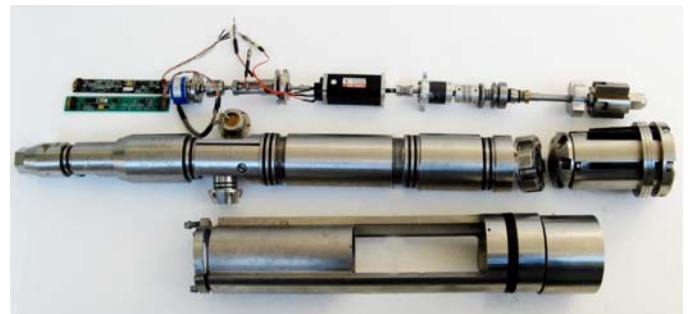
Fig. 1b - Prototype single-siren tool (disassembled).
