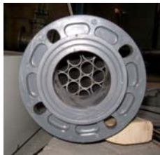
Fig. 5f - Flow straighteners for upstream and downstream use.
