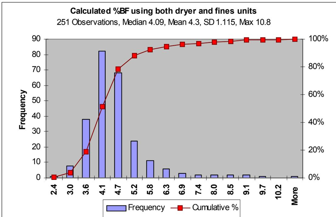
Fig. 3 - Combined ROC Data from Cuttings Dryers and Fines Units.
