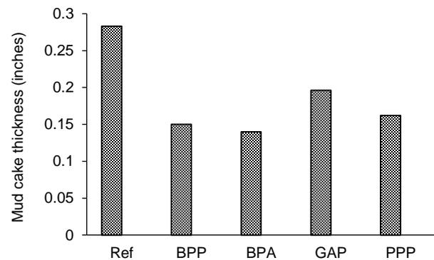
Figure 5. Effect of additives on Mud cake Characteristics
