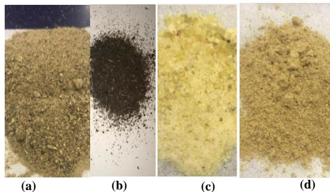
Figure 2. (a) Banana Peels Powder (BPP), (b) Banana Peels Ash (BPA), (c) Gum Arabic Powder (GAP), (d) Potato Peels Powder (PPP)
