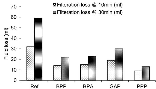
Figure 4. Effect of additives on Filtration loss
