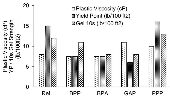
Figure 3. Effect of different additives at 1% concentration on the rheological properties
