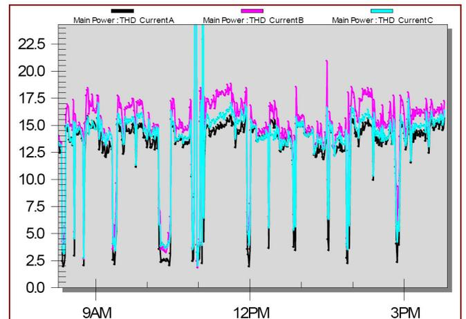
**Figure 2. Measurement of Total Harmonic Distortion (THD) in Position A, B and C in Percentage of Current**
