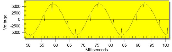
**Figure 1. Example of Voltage Notching**
