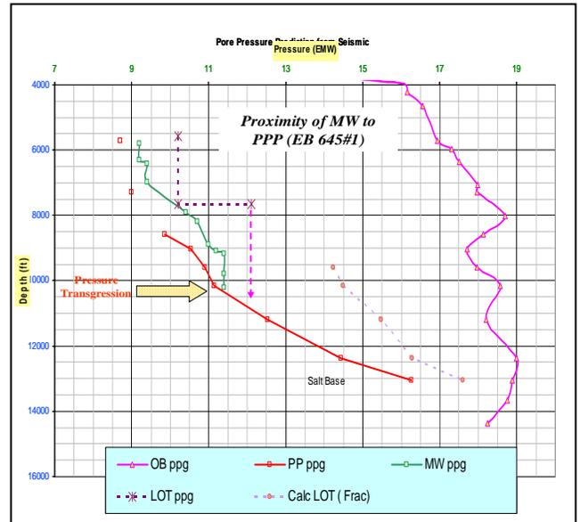
Figure 5: PP plot of EB 645#1 shows the cause of Flow-Kill-Breakdown phenomenon
