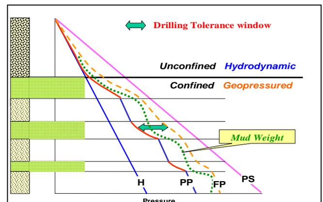
Figure 1: Pressure plot shows the drilling tolerance window
