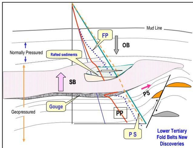
Figure 6: Geopressure model of the salt toe at the Sigsbee Escarpment
