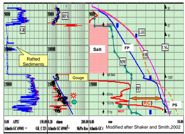
Figure 7: PP plot of GC 699#1 shows the large drop in PP below the salt
