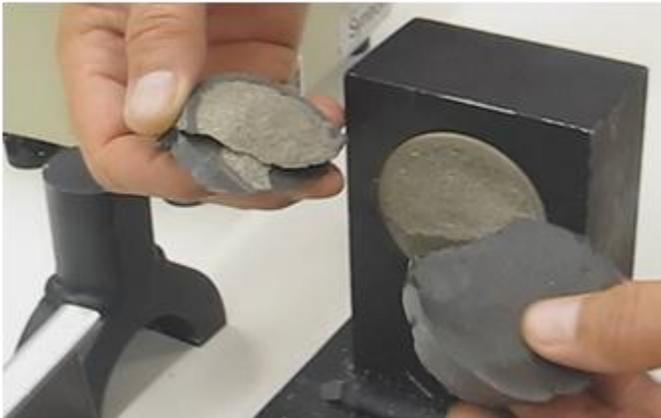
Figure 1: Picture of a post shear strength test showing the fractured surface of the composite core
