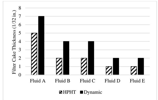
Figure 2- Performance of MDI on filter cake thickness
