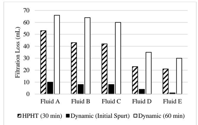
Figure 3-Performance of MDI on filtration loss
