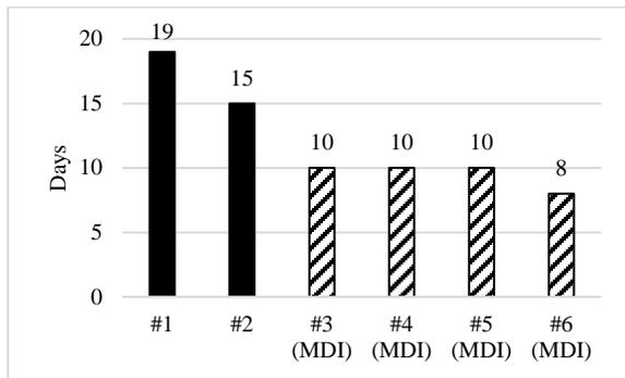
Figure 5-Drilling days (spud to TD) of Howard Well #1-6
