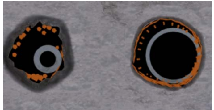
Fig. 4. Wellbore stability improvement by Casing Drilling as compared to conventional drilling.
