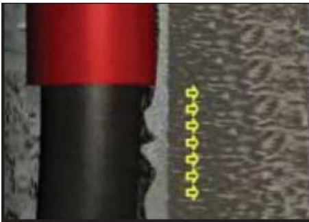
Fig. 3-2. Mud and cuttings are smeared into the formation, while filter cake builds up on the borehole wall.
