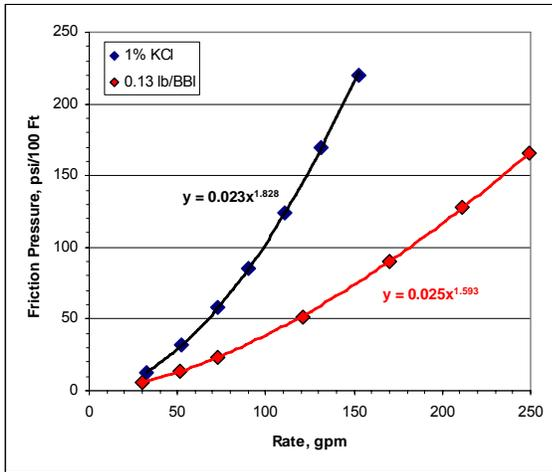
Figure 4 : Effect of 0.13 lb/BBI of the friction reducing polymer on the 1% KCl Brine in 1½ inch coiled tubing.
