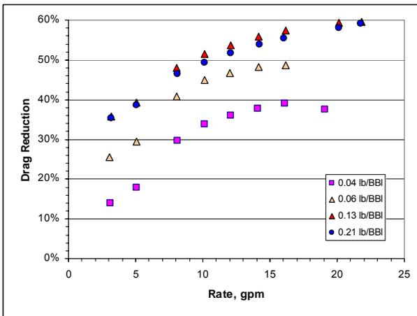
Figure 11 : Drag reduction in coiled tubing for the 10 ppg NaCl brine with varying loadings of Polymer A.
