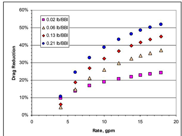
Figure 14 : Drag reduction for 11.4 ppg CaCl<sub>2</sub> brine in coiled tubing, with varying loadings of Polymer A.
