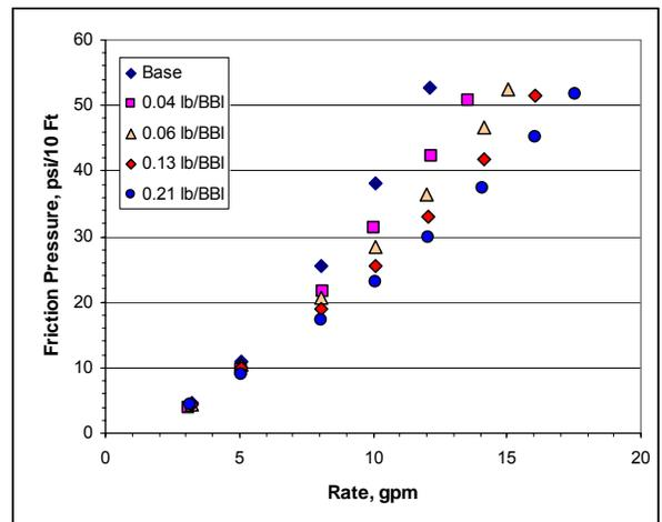
Figure 13: 11.4 ppg CaCl<sub>2</sub> brine in coiled tubing, with varying loadings of Polymer A.
