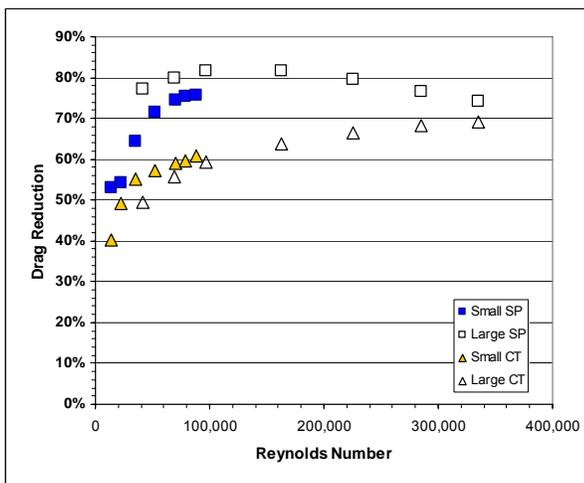
Figure 6 : Drag reduction by 0.06 lb/BBI Polymer A in fresh water in both the large and small scale flow loops. There was good correlation in results between systems for the coiled tubing.
