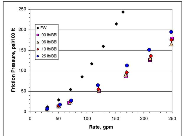
Figure 2 : Friction pressures for fresh water systems in the 1/2 inch coiled tubing.
