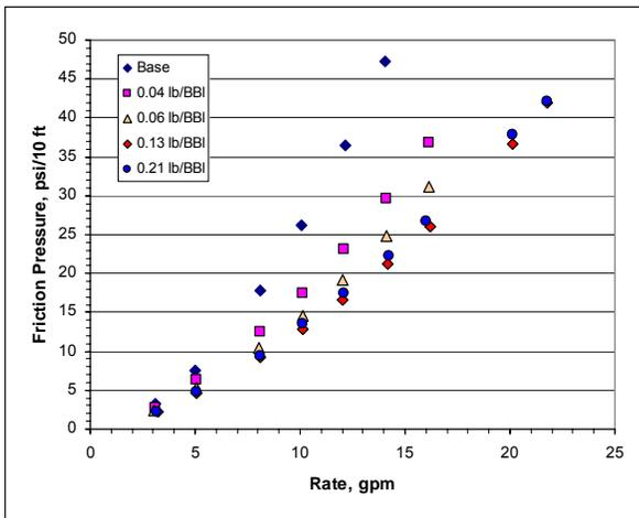
Figure 10 : 10 ppg NaCl brine in ½ inch coiled tubing, with varying loadings of Polymer A.
