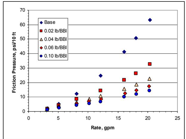
Figure 7 : Friction pressures for 7% KCl in ½ inch straight pipe, with varying loadings of Polymer A.
