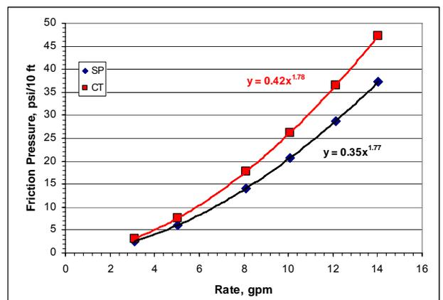
Figure 9 : Base line tests for the 10 ppg NaCl brine. The variation in friction pressure between the coiled tubing and straight pipe was nearly constant at 21%.
