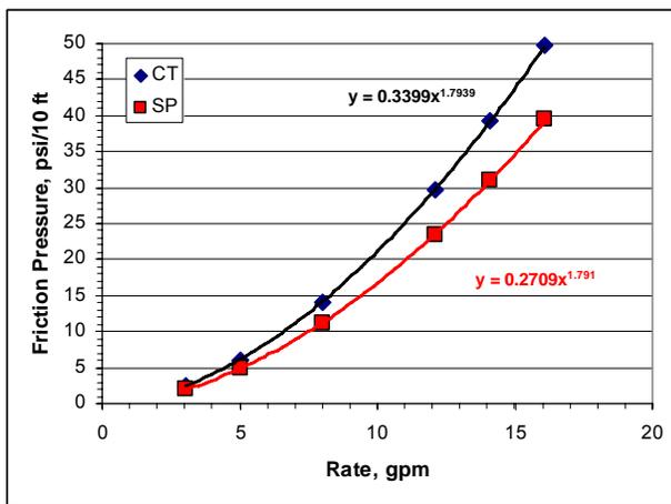
Figure 5 : Fresh water calibration of the small scale (½ inch) flow loop, showing a consistent 21% lower friction in straight pipe than in coiled tubing.
