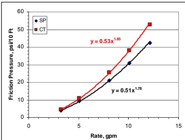
Figure 12 : Base line tests for the 11.4 ppg calcium chloride brine. The difference in friction between the straight pipe and coiled tubing varied from 12% to 20%.
