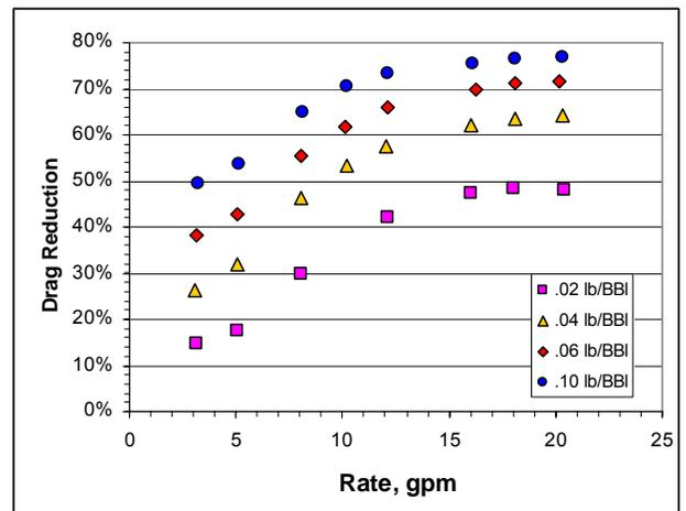
Figure 8 : Drag reduction for Polymer A in 7% KCl in ½ inch straight pipe.
