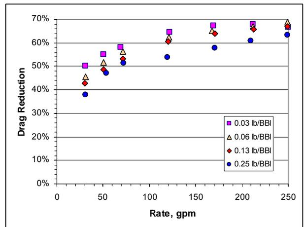
Figure 3 : Drag reduction in 1/2 inch coiled tubing for Polymer A in fresh water.
