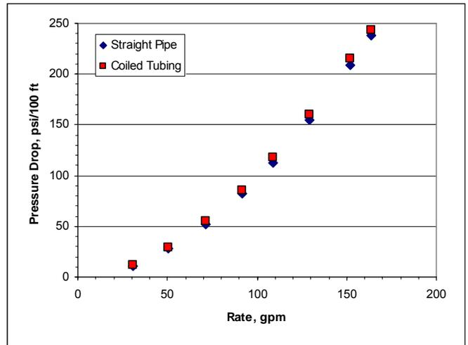
Figure 1 : Fresh water calibration of the 1/2 inch tubing, showing minimal variation between the straight pipe and coiled tubing.
