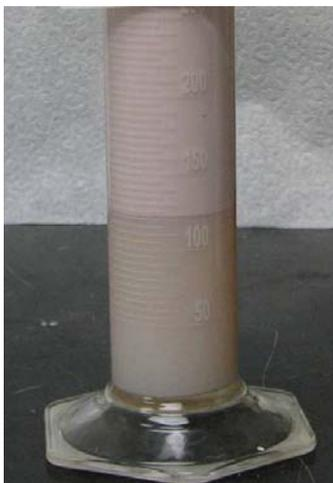
**Figure 4: Emulsifier 1 diesel in saltwater emulsion with viscosifier and fluid loss agent added to the system.**
