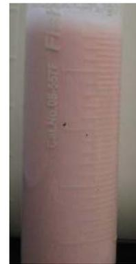
**Figure 7: EP3 diesel in saltwater emulsion with viscosifier and fluid loss agent added to the system after hot-rolling 16 hours at 230°F.**
