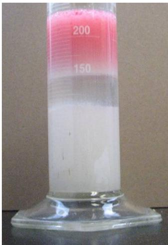
**Figure 10:** EP3 diesel in saltwater emulsion at pH 6 after 8 hours.
