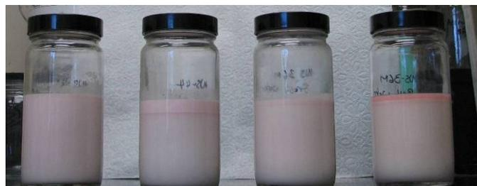
**Figure 1: Emulsifier 2 in freshwater (left) and KCl (left, center) and Emulsifier 1 in freshwater (right, center) and KCl (right).**
