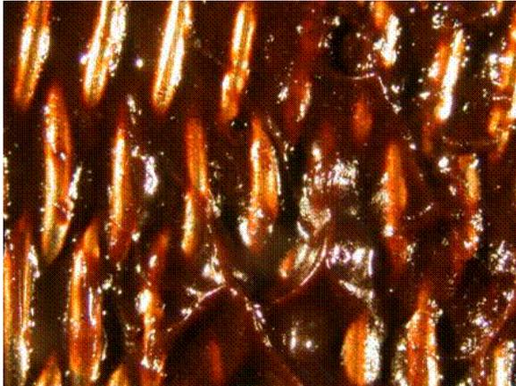
**Figure 7:** Filter cake screen plugging from lab testing (NAF only, no treatment)
