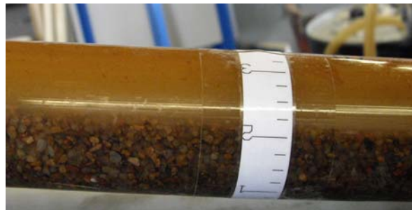
Fig. 2 Example of a bed height measurement along the test section
