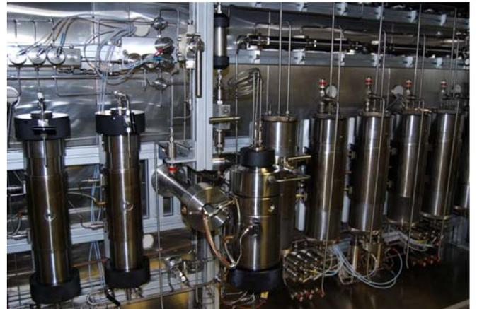
**Fig. 12—Schematic of Hassler Cell Permeameter.**
