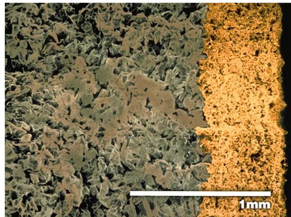
**Fig. 5—Sized Calcium Carbonate viewed with an SEM.**
