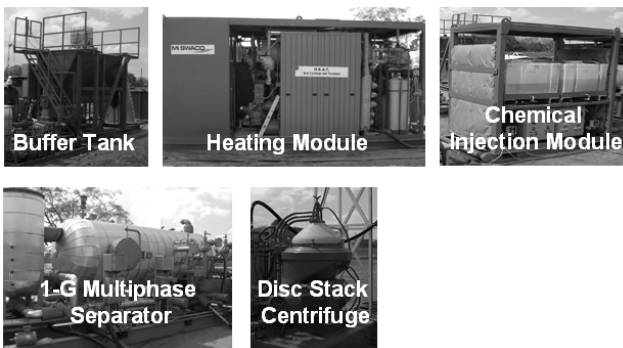
Figure 4 – Equipment Modules Utilized on Location to Treat Production Waste.
