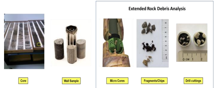
Figure 1. Conventional and Extended Rock Debris Samples
