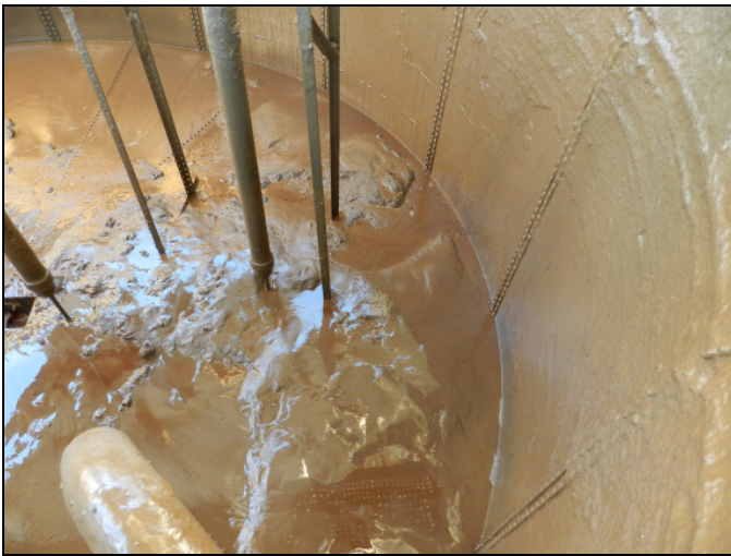
Figure 9: Oil-based mud residue settled in the mixing tank. Areas inside the tank have large sediment deposits accumulated over a period of time.
