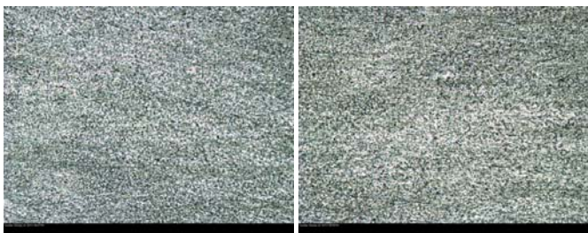
Figure 7: Microscopic photographs at 50X magnification of the two coupon surfaces treated with Chemical A at a dose rate of 2,500 ppm tested in CaCl 2 11.6 PPG
