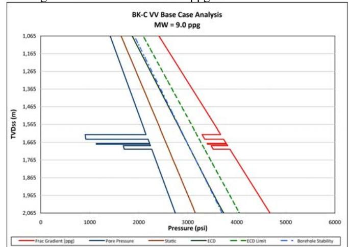
Figure 5. Results of the MPD case analysis for BK-C VV. The modeled ECD is only marginally greater than the wellbore stability making VV drillable with 9.0 ppg MW.
