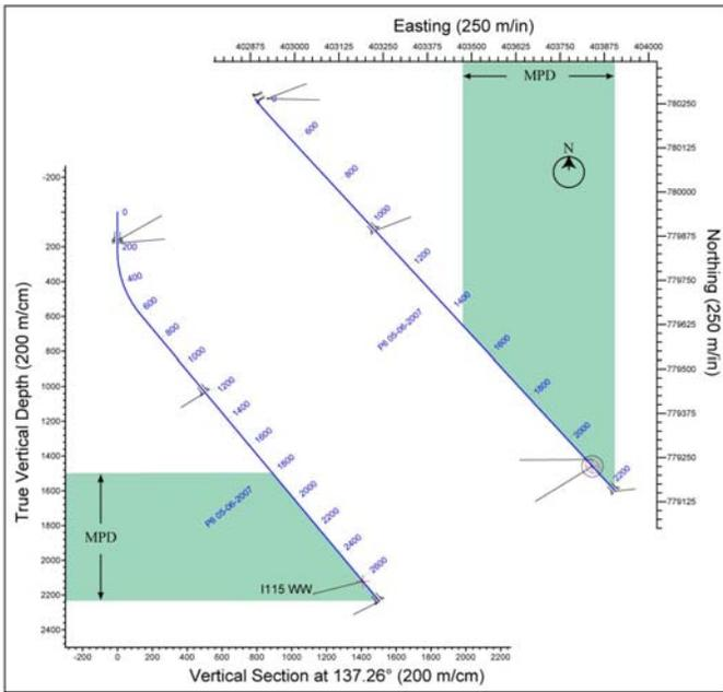
Figure 11. Well plot of BK-C WW showing the tangent section drilled with MPD.
