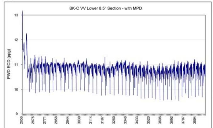
Figure 9. PWD plot in lower 8 1/2" hole section of BK-C VV drilled with MPD and 9.0 ppg static MW. The ECD was kept at or below 11 ppg EMW for the entire section and unlike the upper section it was stable and constant throughout.
