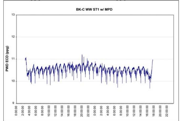
Figure 14. PWD plot in lower 8 1/2 inch hole section of BK-C WW drilled with MPD and 9.0 ppg static MW. The ECD was kept well below 11 ppg EMW for the entire section and it was more stable than the upper section.
