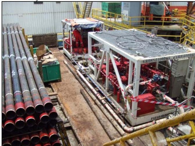
Figure 18. The DAPC choke manifold and backpressure pump rigged up next to the catwalk on the Bunga Kekwa C platform.
