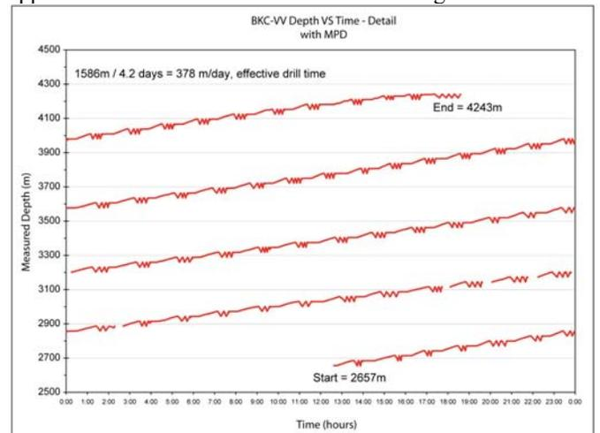
Figure 10. Plot of depth versus time from section of BK-C VV drilled with MPD. Even though the rig continued to back ream each stand 3 times before every connection drilling averaged 378 m/day compared to 275 m/day achieved in the offset well shown in Figure 6.
