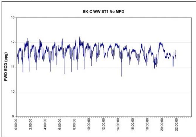
Figure 13. PWD plot in upper 8 1/2 inch hole section of BK-C WW drilled without MPD, with 10.2 ppg static MW. ECD stays
