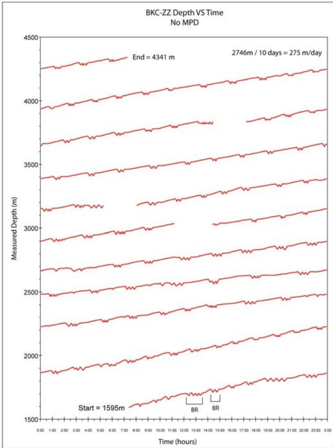
Figure 6. Depth versus time from an offset well showing the non-productive impact of back reaming. Each stand is back reamed 2-3 times, sometimes more, adding 30-60 minutes of flat time which for 80 connections is about 2 days of NPT.
