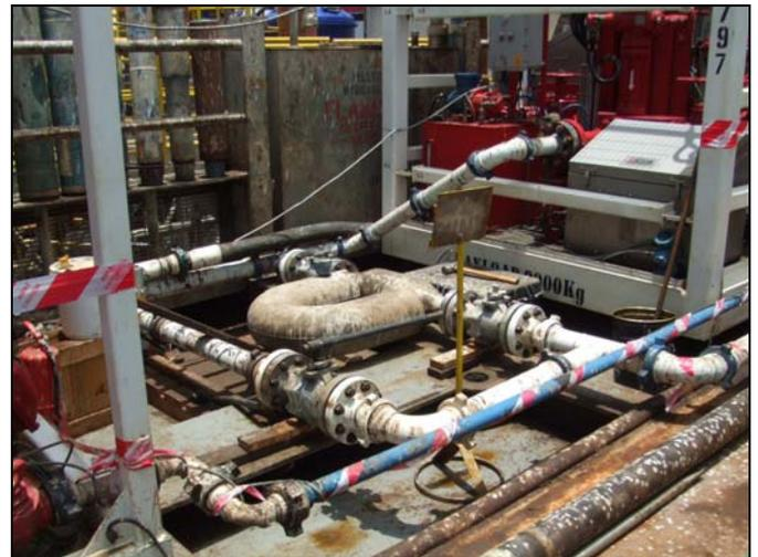
Figure 19. Coriolis flow meter rigged up and connected to the discharge outlet of the choke manifold.
