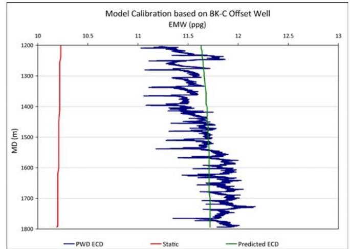
Figure 3. Predicted ECD (green line) for BK-C reference offset well calculated by hydraulics model after calibration.
