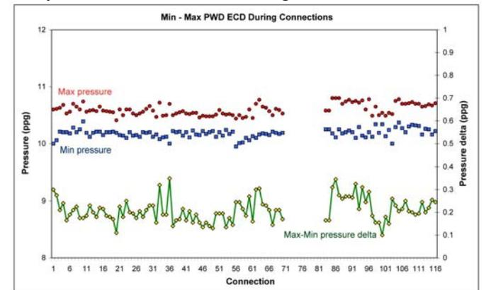
Figure 16. Plot of maximum and minimum pressure recorded on every connection made with MPD in three Bunga Kekwa wells.
