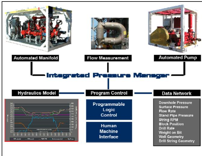
Figure 17. Schematic showing the main components of the DAPC system. The Integrated Pressure Manager consists of the programmable controller, the human machine interface, and the hydraulics mode. The IPM controls the choke manifold and the backpressure pump and monitors flow in and out for early kick detection.
