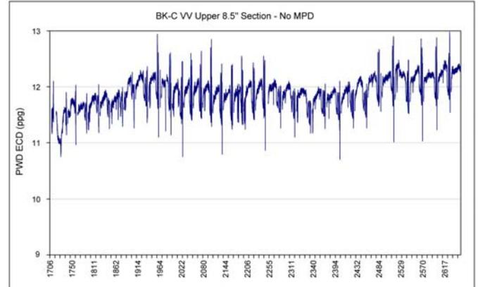
Figure 8. PWD plot in upper 8 1/2" hole section of BK-C VV drilled without MPD, with 10.2 ppg static MW. ECD is unstable throughout and climbs from 11.25 to almost 12.5 ppg.
