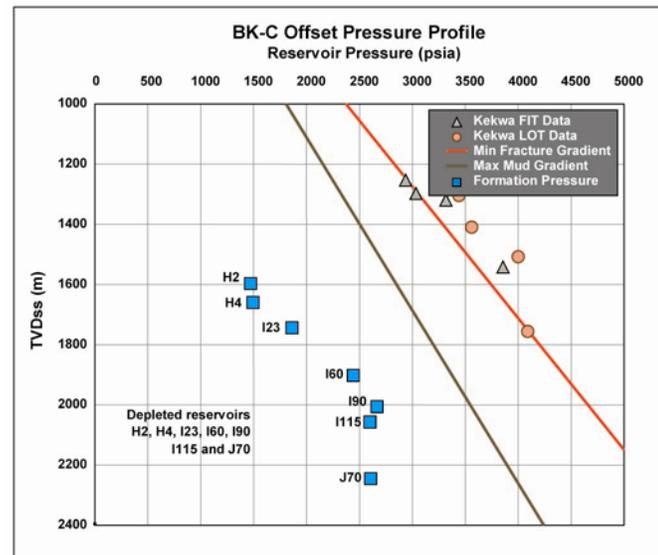
Figure 2. Pressure profile from BK-C reference offset well showing some of the depleted gas sands commonly encountered in the Malay Basin. Total losses occurred in this offset well in the H2 sand.
