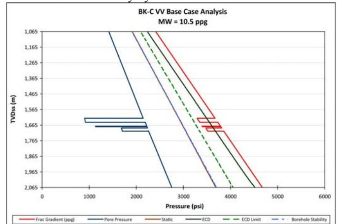
Figure 4. Results of the base case analysis for BK-C VV. The modeled ECD exceeds the fracture gradient in the H2 sand making VV undrillable with 10.5 ppg MW.
