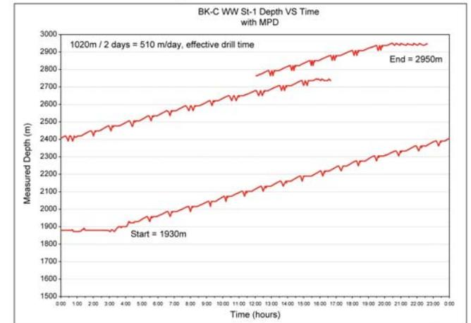
Figure 15. Depth vs. time from section of BK-C WW drilled with MPD. Back reaming was reduced significantly, 1-2 times per stand, and drilling averaged 510 m/day compared to 275 m/day in the offset well shown in Figure 6.
