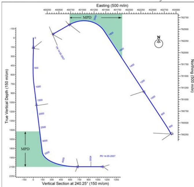
Figure 7. Well plot of BK-C VV showing the angle build and turn section drilled with MPD.
