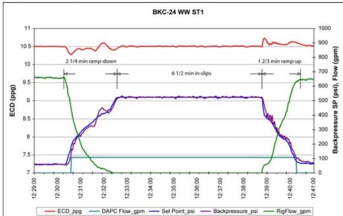
Figure 12. Plot of pressures during a connection made on BK-C WW ST1. In this example, the pump-to-pump connection time is less than 10.5 minutes.
