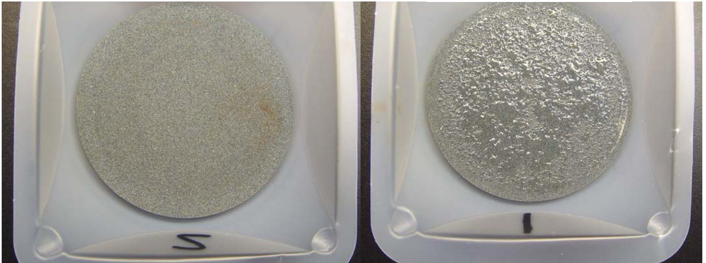
**Fig 8.** Comparison of laboratory cleanup using an HCl-based treatment (left) and an enzyme-based treatment (right). Both RDF systems contained no simulated drill solids.
