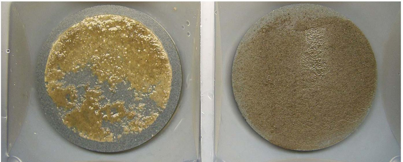
**Fig. 9** - Comparison of laboratory cleanup utilizing an HCl-based treatment (right) and an enzyme-based treatment (left). Both RDF systems contained 2.5% simulated drill solids by volume.
