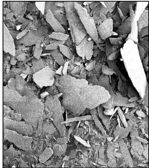
Figure 11 - Calcium carbonate flakes
