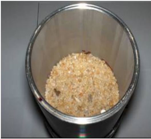
Figure 4 - Filter cell containing the Macae sand
