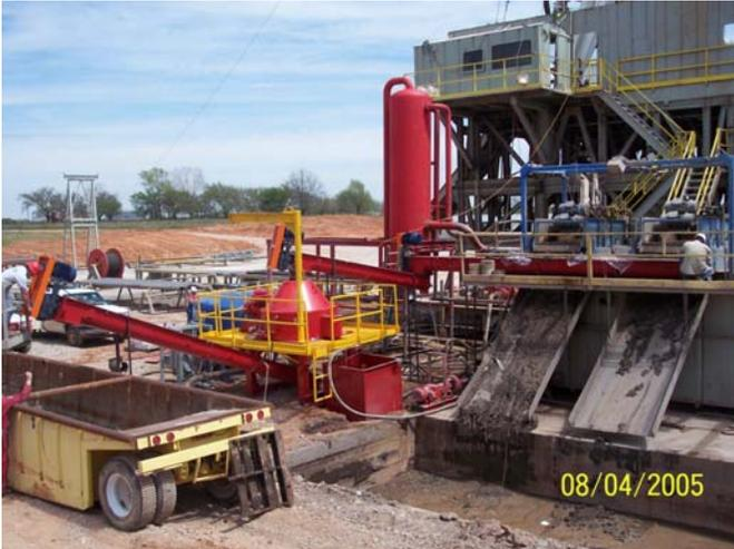
Photograph 1. Standard Vertical Cuttings Dryer Installed on Chesapeake land rig in Oklahoma
