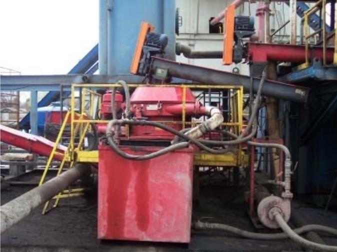
Photograph 5. Small VCD and effluent tank installed on City of Marlow location
