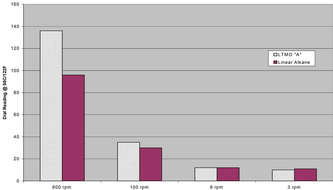
Fig. 2 – Reduction in rheological properties obtainable with low-dispersion emulsifier package in combination with linear alkane base oil in comparison to fluid using conventional package. Both fluids have identical density of 1.68 sg (14.0 lb/gal) and similar OWR.
