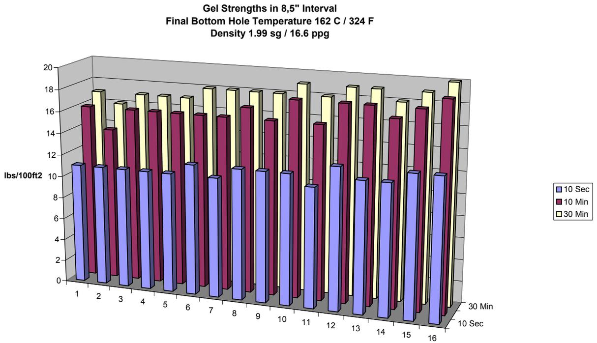
Fig. 4 – Measured gel strengths at 50°C from Norwegian HTHP well.
