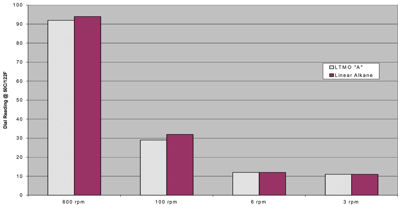
Fig. 1 – Similar rheological properties obtainable with low-dispersion emulsifier package in combination with a linear alkane base oil with an OWR of 75:25 and a density of 1.74 sg (14.5 lb/gal) compared to a conventional system with an OWR of 80:20 and a density of 1.58 sg (13.17 lb/gal).
