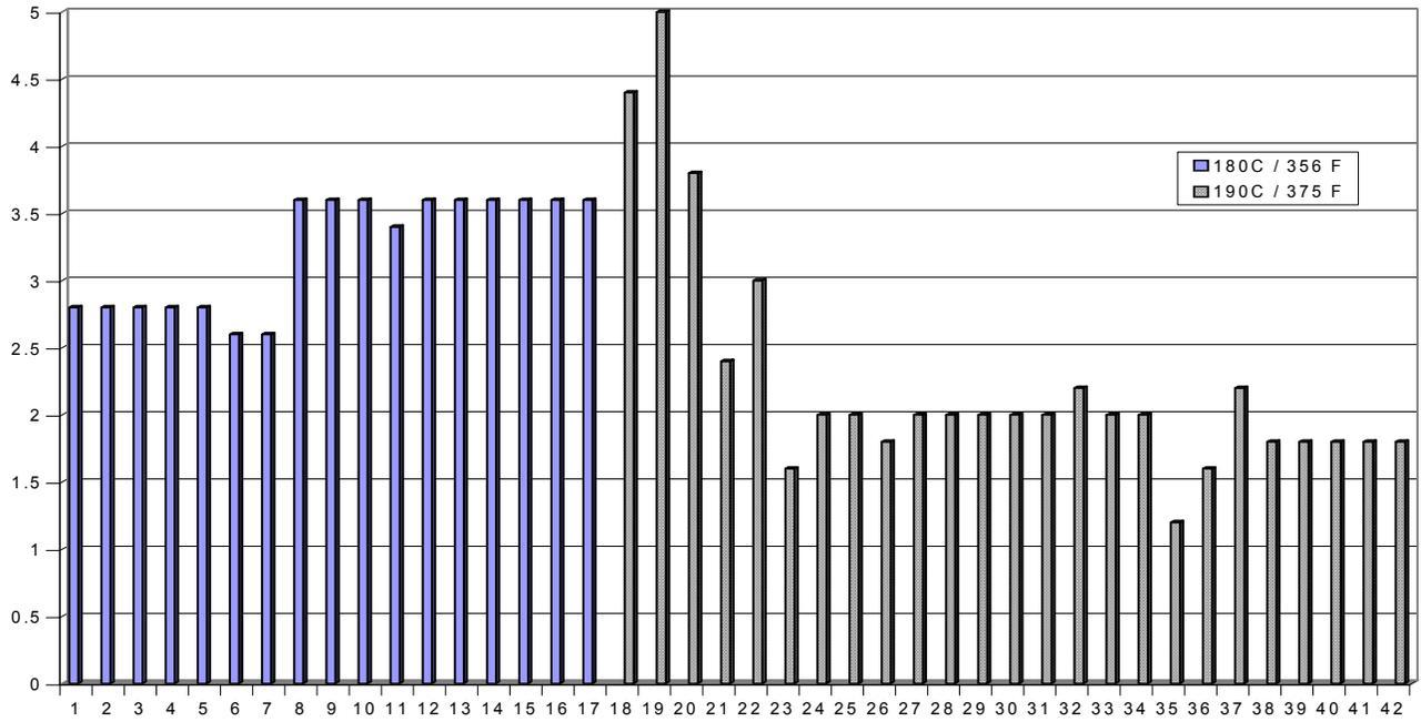
Fig. 3 – HTHP filtrate values measured at 180° and 190°C from Norwegian HTHP well.
