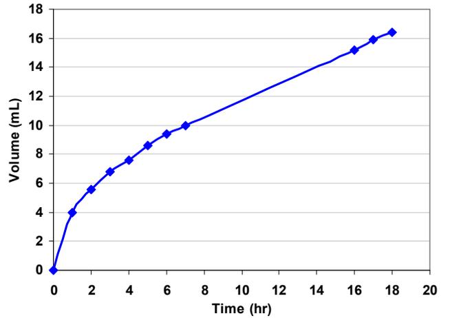
Figure 7 Effect of IEGPF on static filtration
