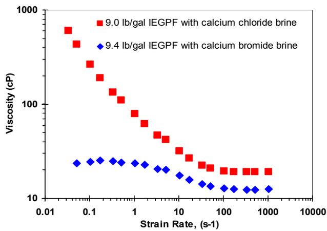
Figure 12 Non-Newtonian behavior of IEGPF with calcium chloride brine
