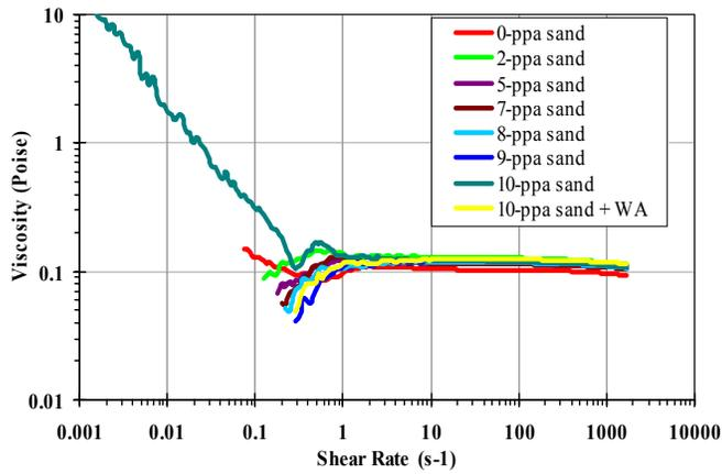
Figure 4 Effect of proppant loading on LSRV
