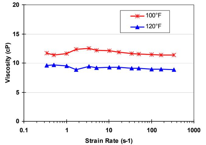
**Figure 1 Low shear rate viscosity of 9.5 lb/gal IEGPF**
