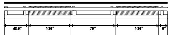
Figure 9 Detail of the Gravel Pack Screen
