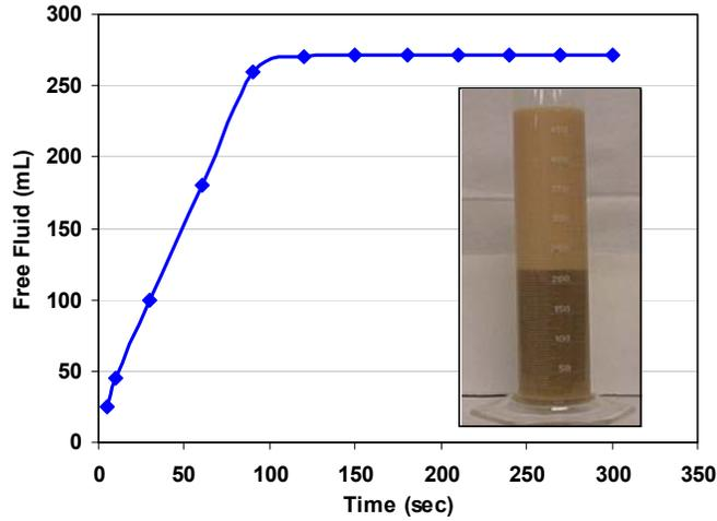
Figure 5 Settling of 20/40 sand in 10.5 lb/gal IEGPF
