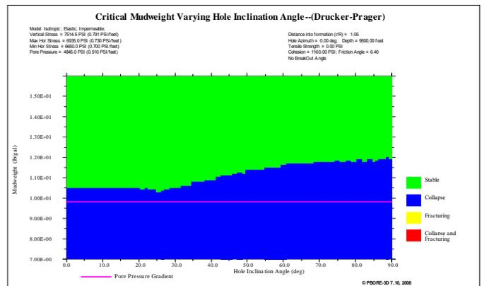
**Fig. 4 – Example of output from software model.**
