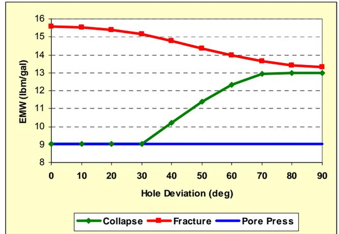
**Fig. 2 – Example of a narrow safe drilling window, North Sea ERD well.**
