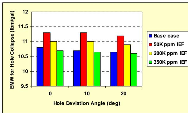
Fig. 6 – EMW to prevent hole collapse for anisotropic deepwater case.
