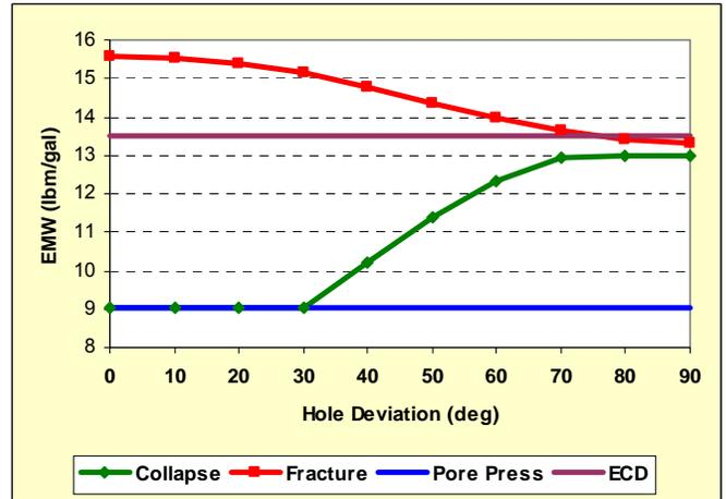
**Fig. 3 – An example of ECD violating the safe drilling window (ECD = 13.5 lbm/gal).**
