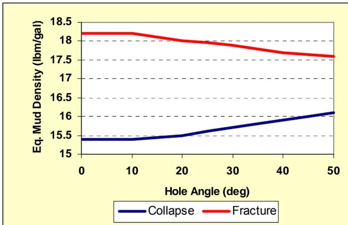
**Fig. 1 – A typical safe drilling window up to 50° deviation.**
