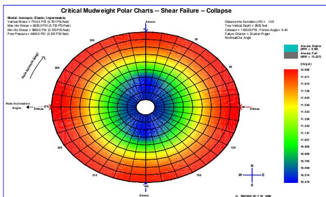
Fig. 7 – Example of output from software model for all possible hole angle and azimuth combinations.
