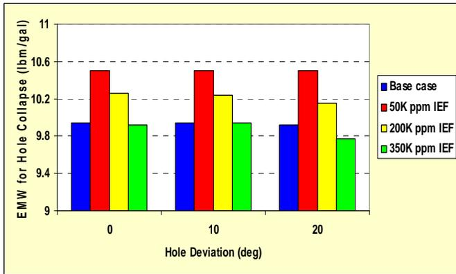
Fig 5 – EMW to prevent hole collapse for isotropic deepwater case.
