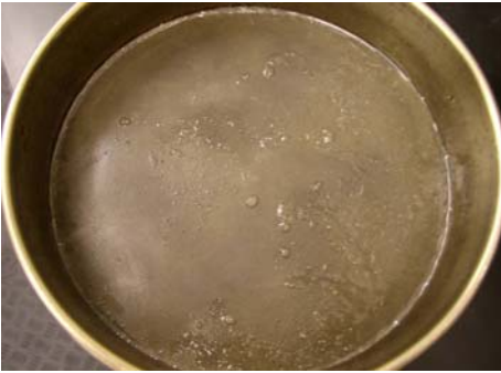
Figure 1. Some fish eyes on the 80-mesh screen after shearing by the single-stage unit.
