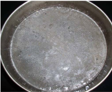
Figure 2. Shows no fish eyes on the 80-mesh screen after shearing by the multi-stage unit.
