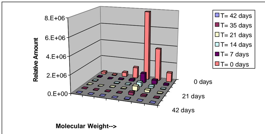
Fig. 5 – Composting trial showing chromatographic analysis of hydrocarbon content of cuttings over a period of 42 days (the seven groups of bars correspond to seven individual components)
