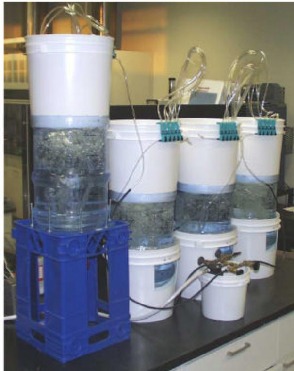
Fig. 1 – Four 15-L Bioreactors
