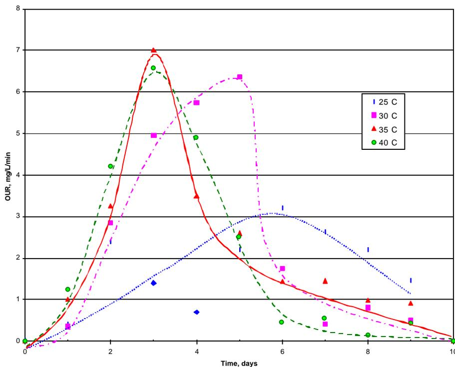
Fig. 3 - Effect of Temperature on Biodegradation Rate in Bioreactor: Formulation N on Simulated Cuttings.
