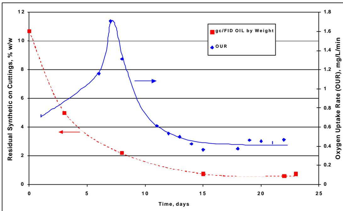
Fig. 2 - Bioreactor Test with Formulation N on Simulated Cuttings: Effect of Time on Oxygen Uptake Rate (OUR) and % Synthetic on Cuttings, 25 °C
