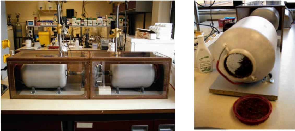
Fig. 4 – Lab scale rotary composter showing encased rotating drums on the left and individual 5-gal drum on the right.
