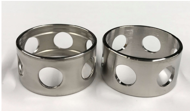
Figure 6. Scratching marks on the inner surface of general purpose disintegration head after shear degradation testing of walnut shell samples. Another lightly used work head was shown (right) for comparison.
