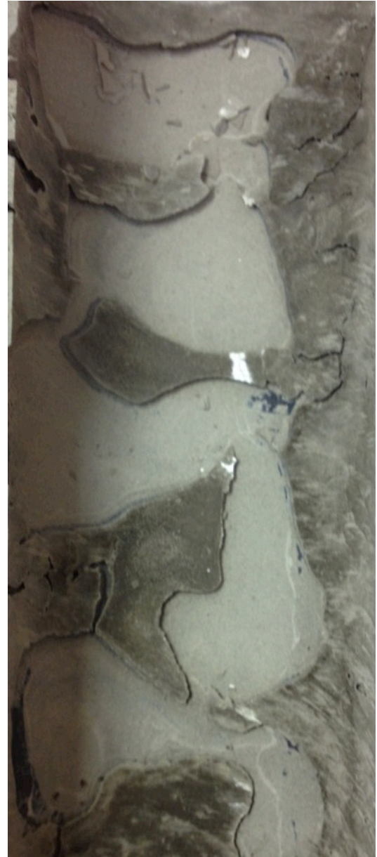
Figure 1: Cement Channeling in Lab
