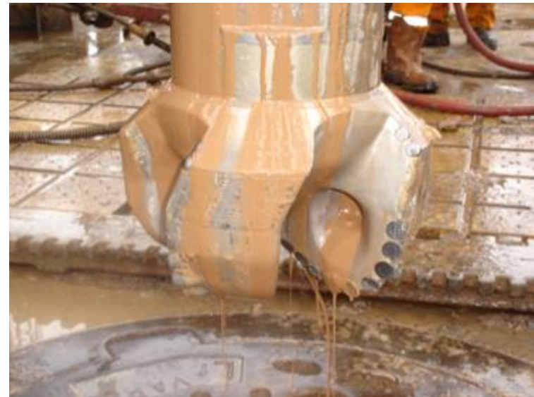
Figure 3 –PDC bit WELL #1 with HPWBM on WELL #1
