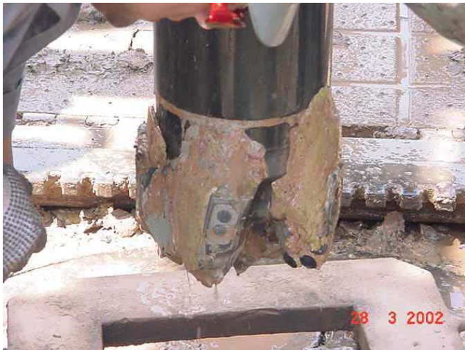
Figure 2 –PDC bit from offset wells with conventional WBM
