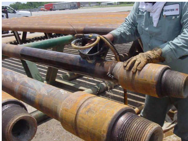
UT hand scanning critical areas with multiple probes
