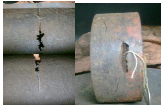
Washouts occurring from non-routine inspecting programs
