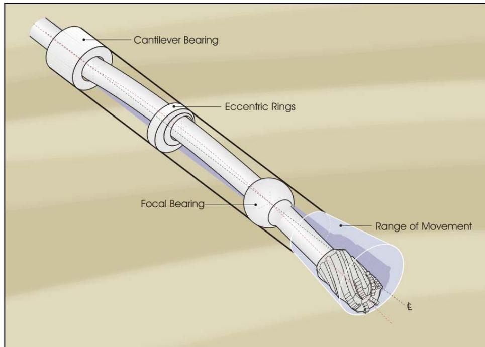
Fig 3. A points to Bit Rotary Steerable Tool Concept (Cited from Tetsuo, et al. [1])
