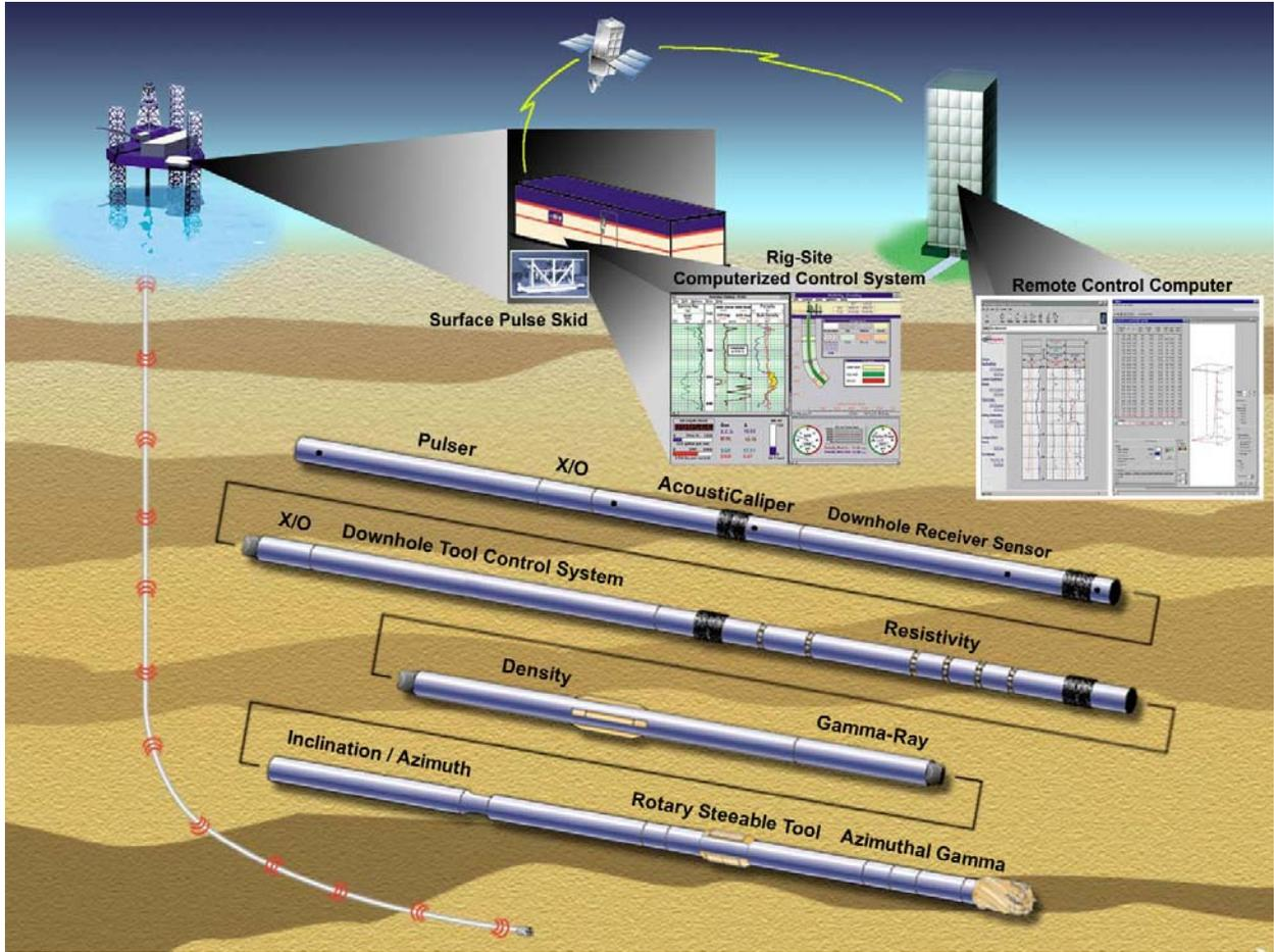
Figure 1. Downlink Drilling Control System and Downhole BHA Integration (adapted from Tetsuo, et al. [1])
