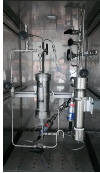
Figure 5 – (right) Photograph of PTT equipment in a controlled temperature environment, showing sample core holder with an upstream and downstream fluid reservoir that allows for pressure transmission through a cylindrical shale sample to be measured; (below) example of test result, with downstream pressure data processed in accordance with Eq.(2) and fitted with a least-squares linear fit. From the slope of the fitted lines obtained for the pore fluid (first) cycle and the test fluid (second) cycle, a delay factor can be characterized according to Eq.(3). The delay factor is a quantitative measure for the available trouble-free open hole time expected with the test fluid in the shale borehole.
