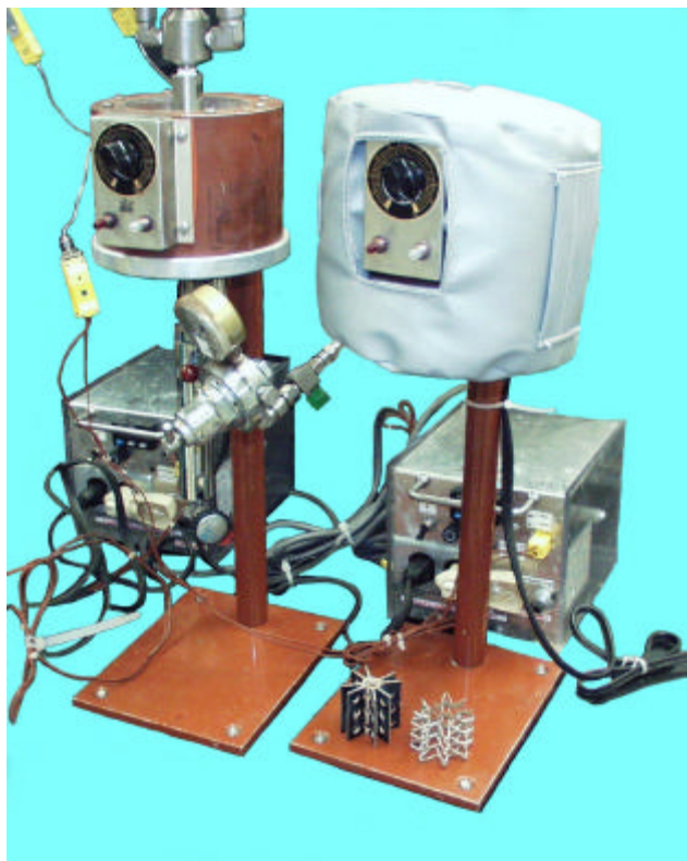
Figure 4 - Jacket insulation, heat sinks, and jacket heating controllers
