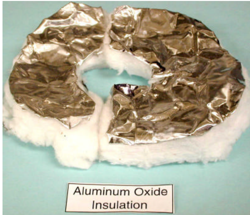
Figure 16 – Aluminum oxide top insulation for 250-mL cell
