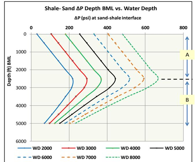
**Figure 8:** Plot exhibits the sand-shale differential pressure (psi) vs. depth below the mud line for several water depth setting ranges from 2,000 ft to 8,000 ft (SS). The possible depth of zones A - B contact ranges from 2,000 ft to 3,000ft.
