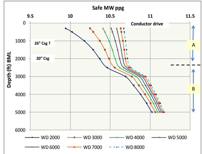
**Figure 10:** A plot represents the safe mud weight required to drill the section between the base of the conductor to the surface casing and beyond in different water depth. Safe MW is reference to depth BML and WD.
