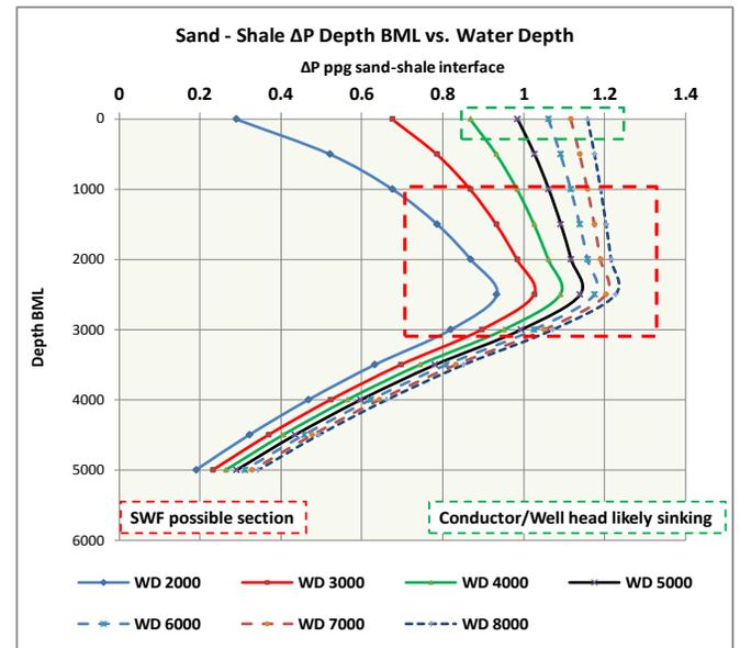
**Figure 9:** Shows the same data on figure 8 converted to ppg mwe. An overbalance MW of 0.8 to 1.2 ppg is required to drill in water depth exceeds 4,000 ft. Moreover, the +/- 300 ft top soil section displays large  $\Delta P$  in water deeper than 5,000 ft (where conductor subject to sink).
