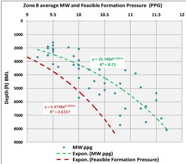
**Figure 7:** Recorded data of mud weight (MW) used to drill several wells in zone B of the GOM deep water. They are from Mississippi Canyon, Green Canyon, and Garden Banks areas respectively. Note the MW increases with depth to combat the increase of the hydrodynamic pressure gradient. The average MW and feasible formation pressure (FFP) calculations of the entire collected data set in ppg below the mud line.
