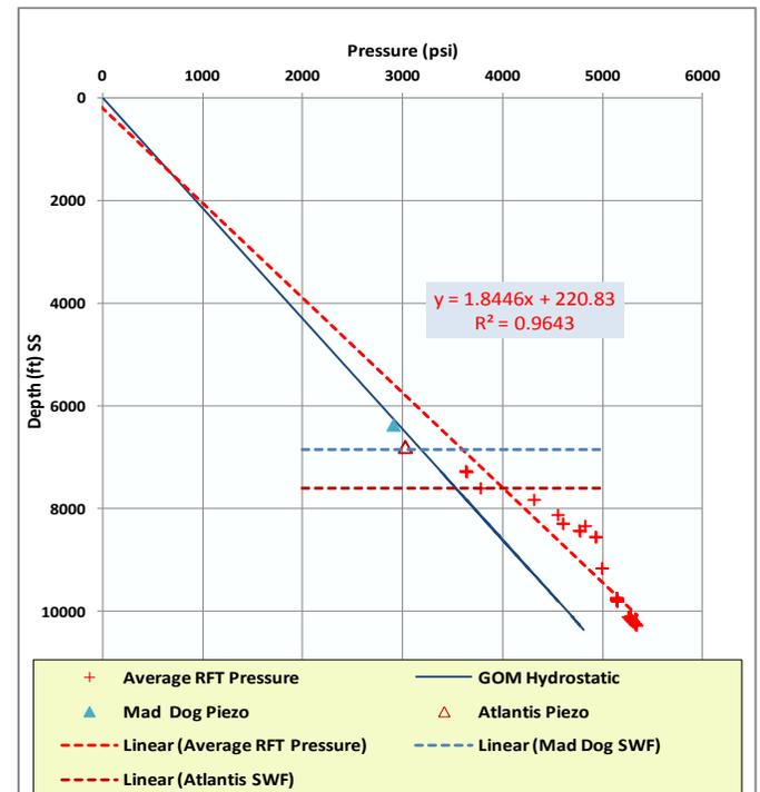
**Figure 6:** Show the same measured pressure data (RFT-MDT) on figure 5 to be plotted in reference to the sea level (SS). Piezoprobe data from Atlantis and Mad Dog are added. An average linear trend ( $R^2 = 0.96$ ) with a pressure gradient of 0.54 psi/ft. Moreover, the resulting hydraulic head (intercept at 0 pressures) is about 220 ft below the sea level. Therefore, water in sand can flow above the mud line for great heights contingent on the water depth.
