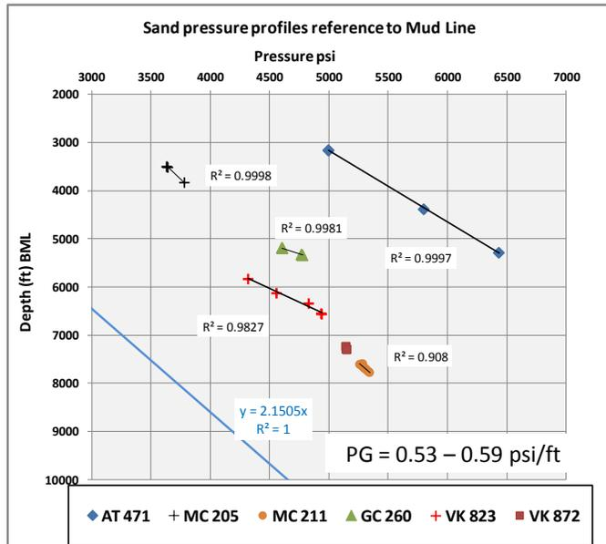
**Figure 5:** Exhibits zone B measured sand pressure (psi) vs. BML depth plot of several wells. The pressure gradients (trend slope) range from 0.53 to 0.59 psi/ft. They show a higher gradient than the GOM hydrostatic gradient (blue trend on the left). They are in non-alliance positions due to the drastic changes of the sea floor topography.
