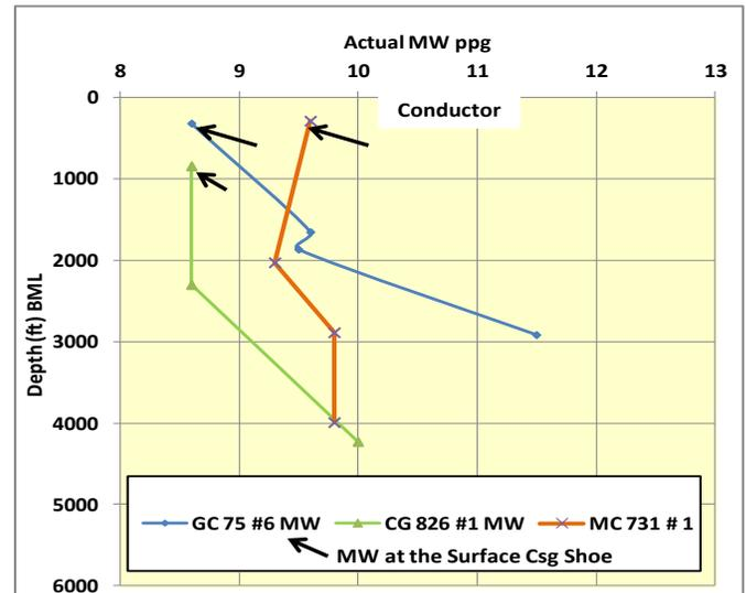
**Figure 11:** Exhibits some of the early deepwater wells (with SWF) that had used the shelf light mud programs (8.5 to 9.5 ppg) to drill to the surface casing shoe. SWFs were costly to overcome.
