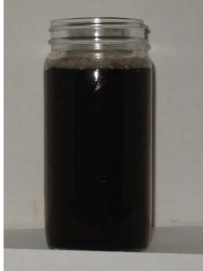
Figure 6. 9.5 lb/gal NaCl after Aging at 300 °F for 16 hours with Oxygen Scavengers
