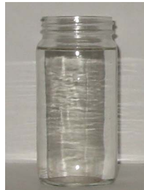
Figure 6. 9.5 lb/gal NaCl after Aging at 300 °F for 16 hours with Oxygen Scavengers
