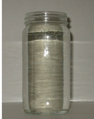
Figure 10. 12.5 lb/gal NaBr after Aging at 300 °F for 16 hours with Oxygen Scavengers
