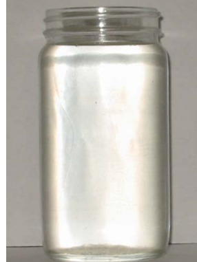
Figure 12. 15.5 lb/gal ZnBr 2 /CaBr 2 after Aging at 300 °F for 16 hours with Oxygen Scavengers
