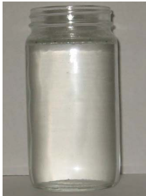
Figure 13. 15.5 lb/gal ZnBr 2 /CaBr 2 after Aging at 400 °F and 500 °F with the New Scavenger
