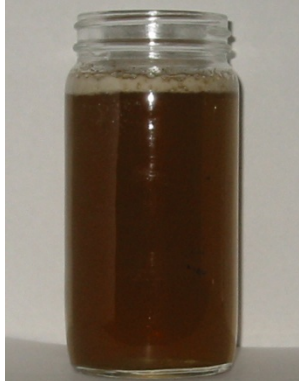
Figure 8. 11.0 lb/gal CaCl 2 after Aging at 300 °F for 16 hours with Oxygen Scavengers
