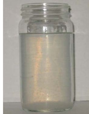
Figure 7. 9.5 lb/gal NaCl after Aging at 400 °F and 500 °F with the New Scavenger
