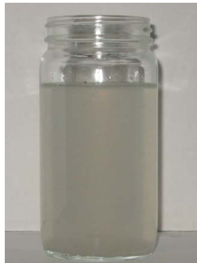
Figure 9. 11.0 lb/gal CaCl 2 after Aging at 400 °F and 500 °F with the New Scavenger
