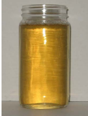
Figure 12. 15.5 lb/gal ZnBr 2 /CaBr 2 after Aging at 300 °F for 16 hours with Oxygen Scavengers
