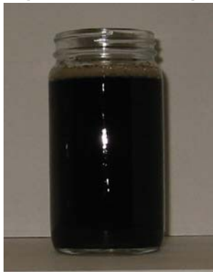
Figure 10. 12.5 lb/gal NaBr after Aging at 300 °F for 16 hours with Oxygen Scavengers
