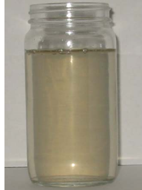
Figure 11. 12.5 lb/gal NaBr after Aging at 400 °F and 500 °F with the New Scavenger
