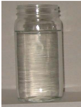
Figure 7. 9.5 lb/gal NaCl after Aging at 400 °F and 500 °F with the New Scavenger
