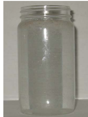
Figure 13. 15.5 lb/gal ZnBr 2 /CaBr 2 after Aging at 400 °F and 500 °F with the New Scavenger
