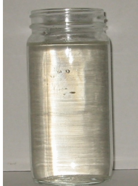
Figure 8. 11.0 lb/gal CaCl 2 after Aging at 300 °F for 16 hours with Oxygen Scavengers
