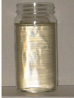
Figure 11. 12.5 lb/gal NaBr after Aging at 400 °F and 500 °F with the New Scavenger
