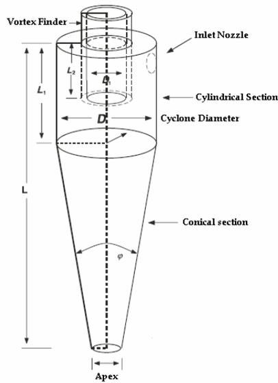
Figure 1. Components of a typical hydrocyclone.
