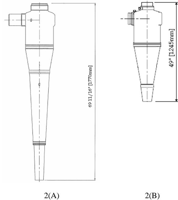
Figure 2. (A) HP 10" hydrocyclone vs. (B) standard 10" hydrocyclone.
