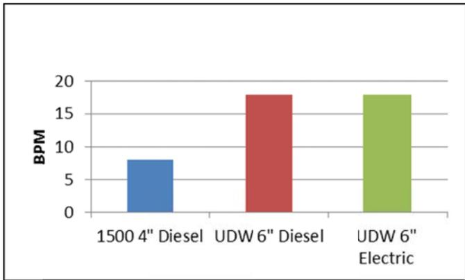
**Figure 1 – Field Trial - High Turbidity Maximum Flow Rates**
