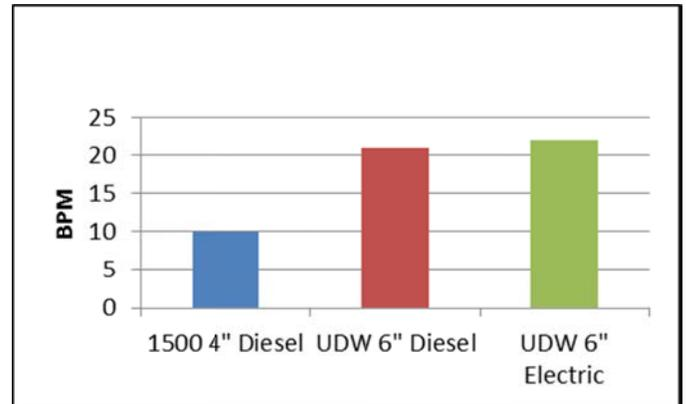
**Figure 2 – Field Trial - Low Turbidity Maximum Flow Rates**
