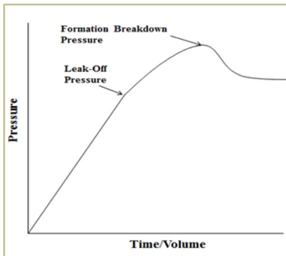
Figure 1. Schematic illustration of pressure-time/volume plot in a leak-off test.
