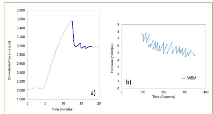
Figure 6. Wave-like pattern pressure drop with fracture propagation. a: field test (after Okland et al.<sup>9</sup>), b: lab test (after Morita et al.<sup>10</sup> and Fuh et al.<sup>11</sup>).
