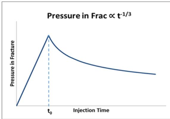
Figure 8. Theoretical prediction of fracture propagation pressure decrease with injection time.
