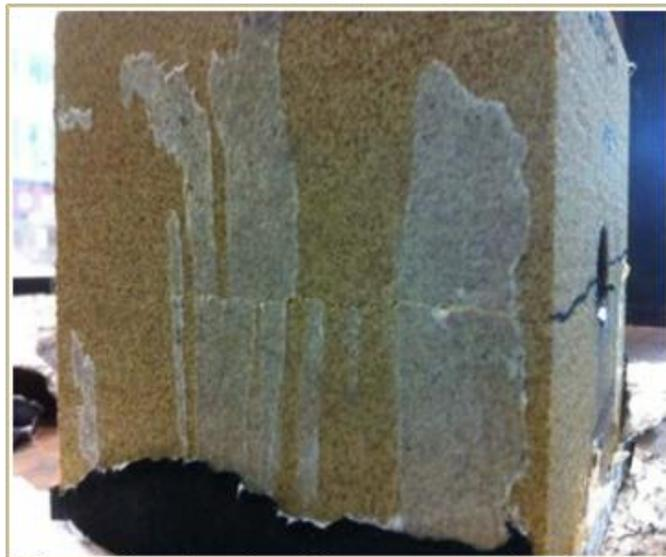
Figure 13. The sandstone test block for pressure build-up curve in Figure 12. The block was fractured to the edges without obvious fluid leak-off due to LCM sealing effect (after Guo, et al.<sup>8</sup>).
