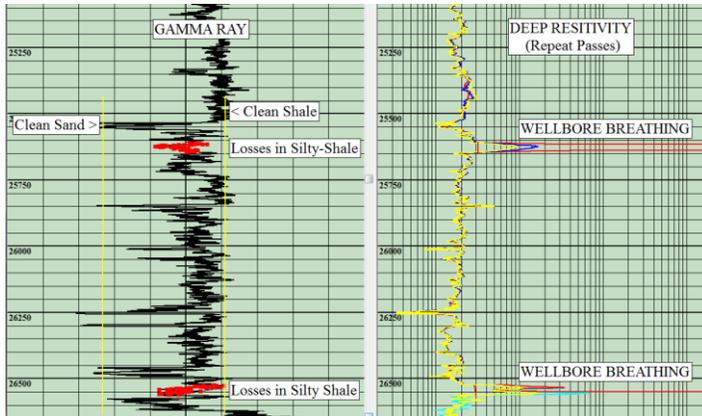
Figure 16. Two lost circulation and wellbore breathing events occurred in silty shale formations, rather than in clean shale or clean sand formations<sup>14, 15</sup>.
