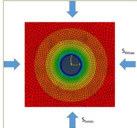
Figure 2. Near wellbore hoop stress concentration with uniform far-field stresses  $S_{Hmin}=S_{Hmax}$  (blue color = more compression, red color = less compression).
