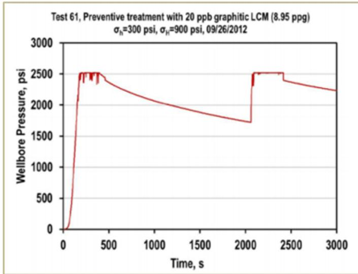
Figure 12. An example of a preventive wellbore strengthening test on a sandstone block (after Guo, et al.<sup>8</sup>).
