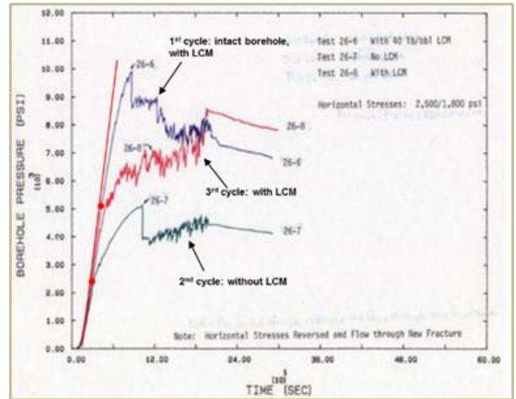
Figure 14. A repeated hydraulic fracturing test with LCM. 1st injection cycle (preventive treatment - intact wellbore, with LCM): high leak-off pressure and high propagation pressure. 2nd injection cycle (fractured wellbore, without LCM): low leak-off pressure and low propagation pressure. 3rd injection cycle (fractured wellbore, with LCM): low leak-off pressure, high (increased) propagation pressure. (after Black et al.<sup>13</sup>).
