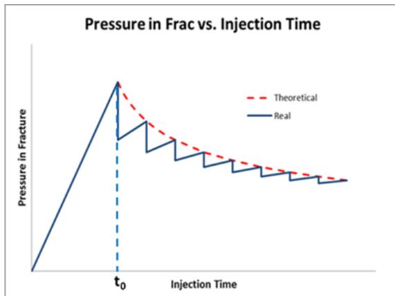
Figure 11. Fracture propagation decrease during injection (blue solid line: real case; red dot line: theoretical prediction).
