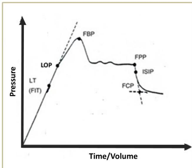
Figure 3. Typical XLOT plot (Modified after Gaarenstroom et al.<sup>4</sup>).
