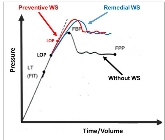
Figure 15. Preventive wellbore strengthening treatment enhances both leak-off pressure and fracture propagation pressure, while remedial wellbore strengthening treatment only enhances fracture propagation.
