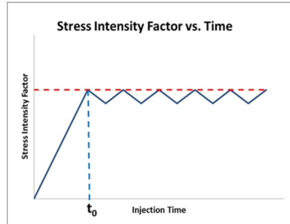
Figure 9. Change of stress intensity factor with injection.
