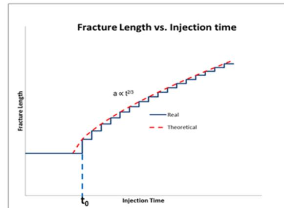
Figure 10. Fracture length increase during fracture propagation (blue solid line: real case; red dotted line: theoretical prediction).
