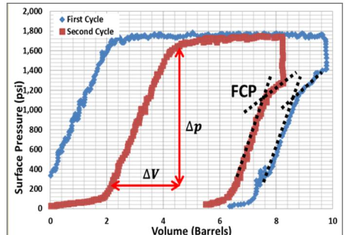
Figure 4. An example of pressure-volume plot in a pump-in and flow-back test (Modified after Gederaas and Raen<sup>5</sup>).
