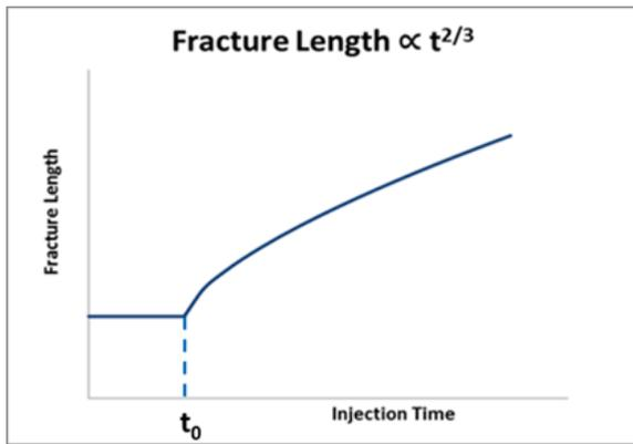
Figure 7. Theoretical prediction of fracture length increase with injection time.
