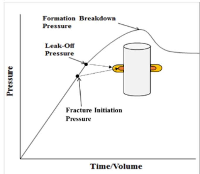
Figure 5. Leak-off pressure is higher than fracture initiation pressure with high solids-content injection fluid, due to mud cake sealing effect.
