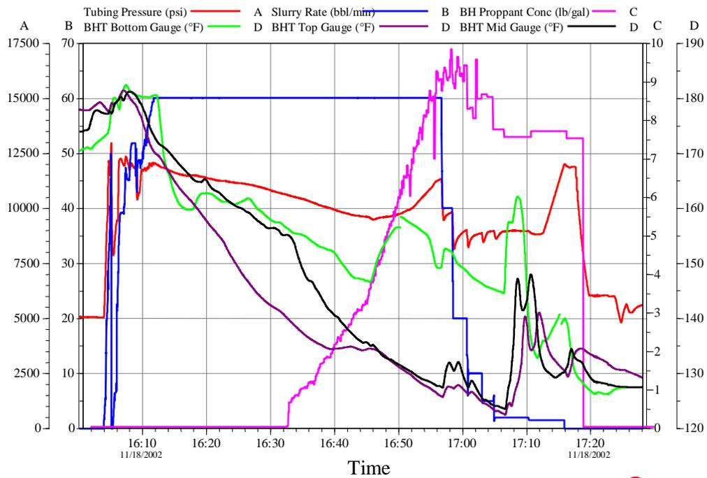
Fig. 11 — Data for the fracpack treatment
