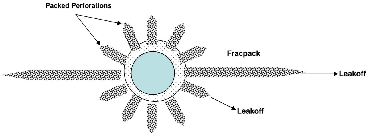
Fig. 5 — Radial View of Leakoff After Screenout
