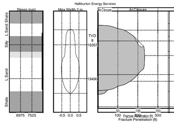
Fig. 12 — Estimated Geometry for the Zone
