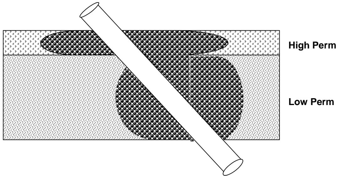
**Fig. 3 — Possibility of Screenout Due to High Permeability Zones**
