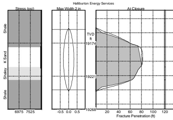
Fig. 16 — Calculated Geometry of FracPac for the Case History 3
