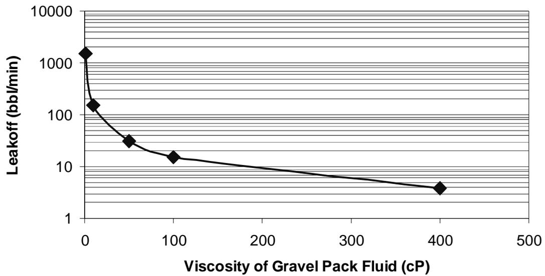
Fig. 6 — Leakoff through a set of packed perforations as a function of the fluid viscosity
