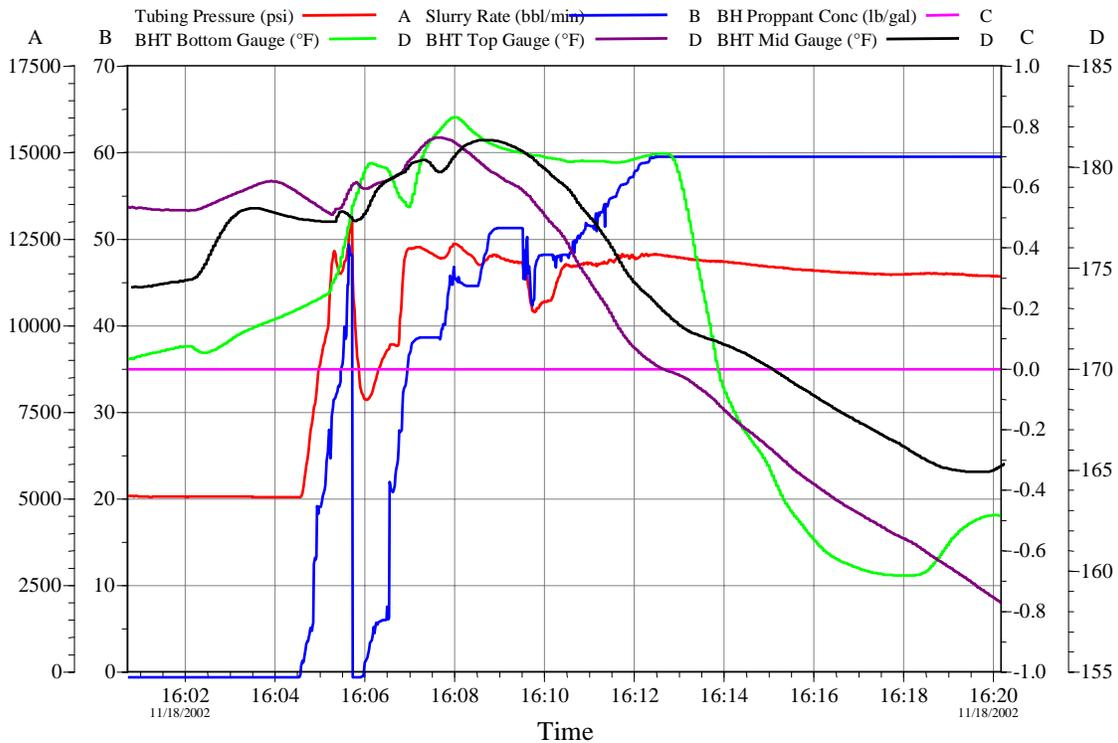
Fig. 10 — Early Time Data for the Main Fracpack Treatment
