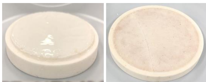
Figure 3 – Filter cake breaker test results before and after 7 day soak period
