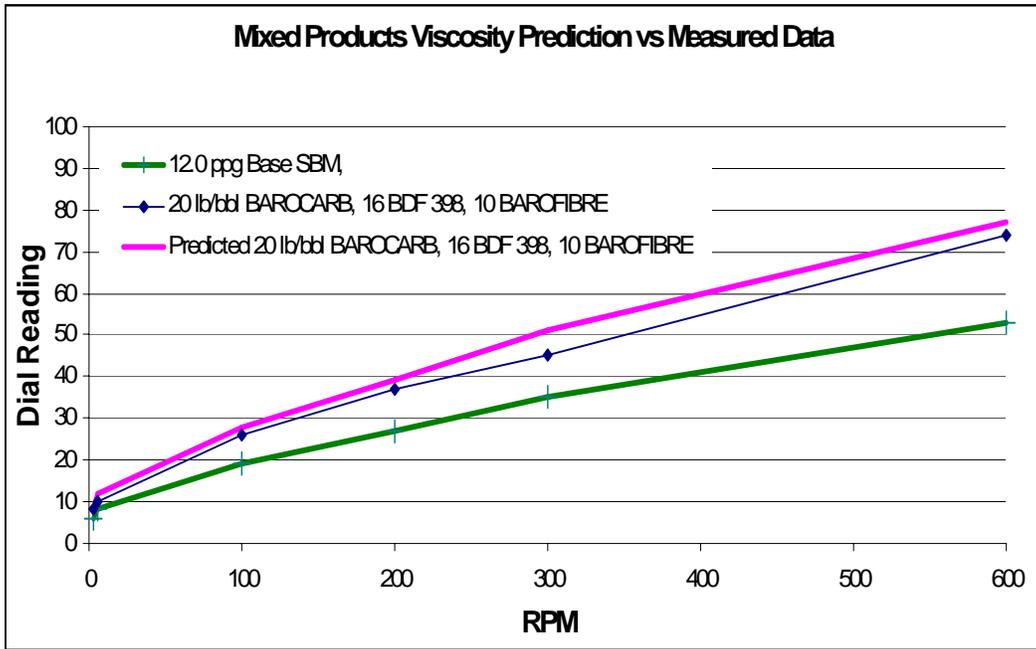
Figure 6 Comparison of Measured Viscosity and Predicted Viscosity for a Particulate Formulation
