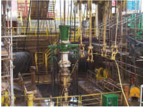
Fig. 5a – RiserCap™ Configuration offshore Brazil (Source: Lage et al, SPE 71361)
