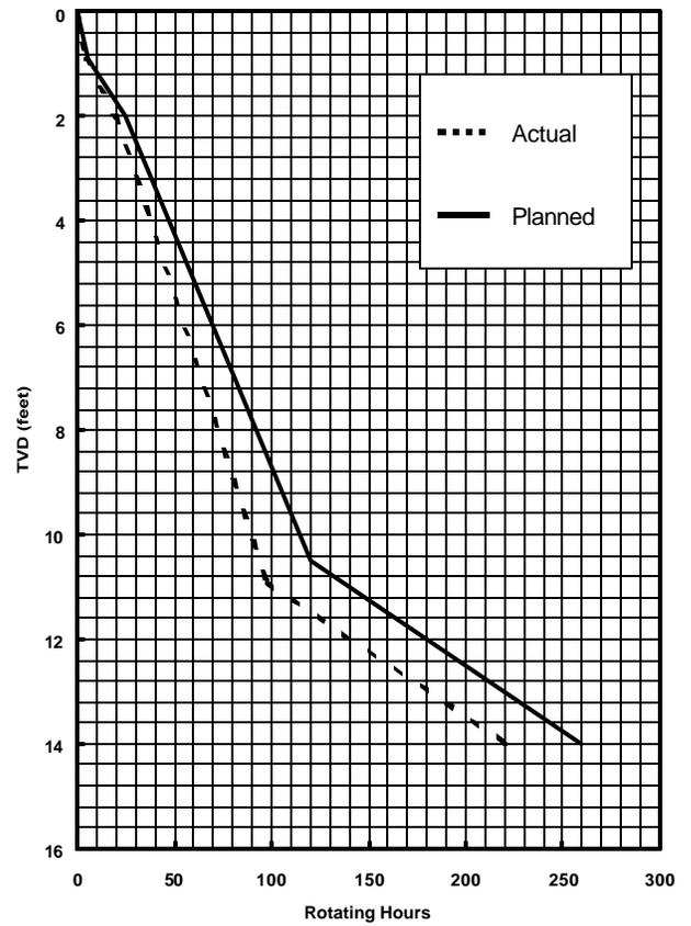
Figure 14. West Delta Rotating Hours Curve
