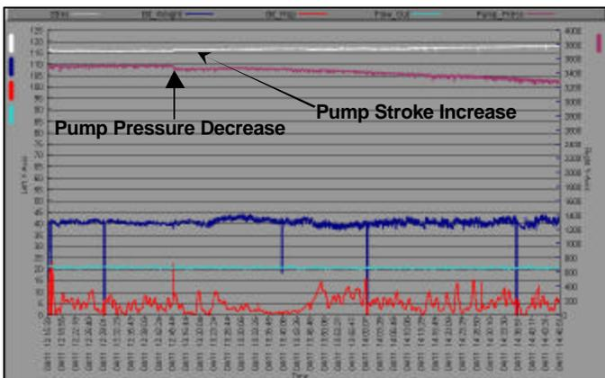
Figure 11. Drill graph event recognition screen. This screen is evidencing a drill pipe washout.
