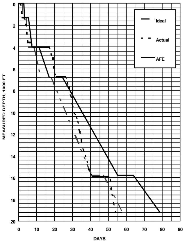
Figure 16. Grand Isle Rotating Hours Curve
