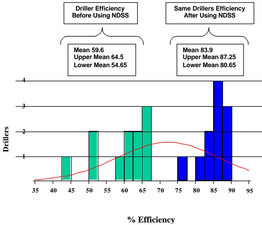
Figure 10. Drilling with and without NDSS
