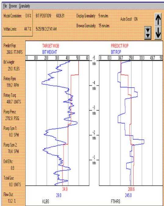
Figure 8. Drilling without NDSSO
