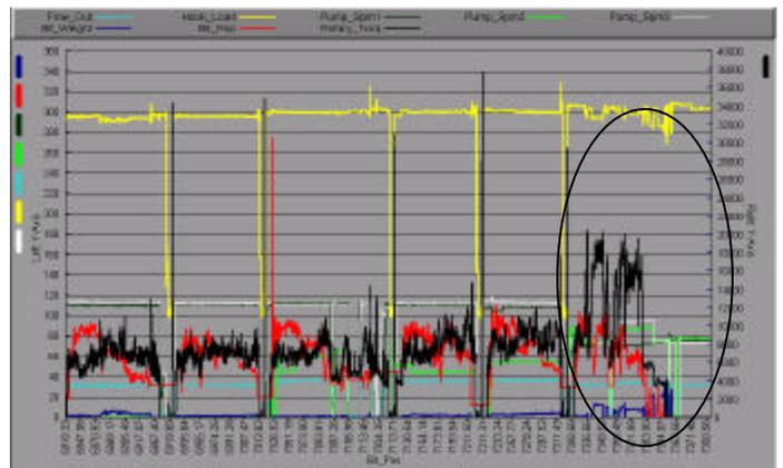
Figure 12. Drill graph event recognition screen. This screen is evidencing a mud motor failure and subsequent twist off after a connection.
