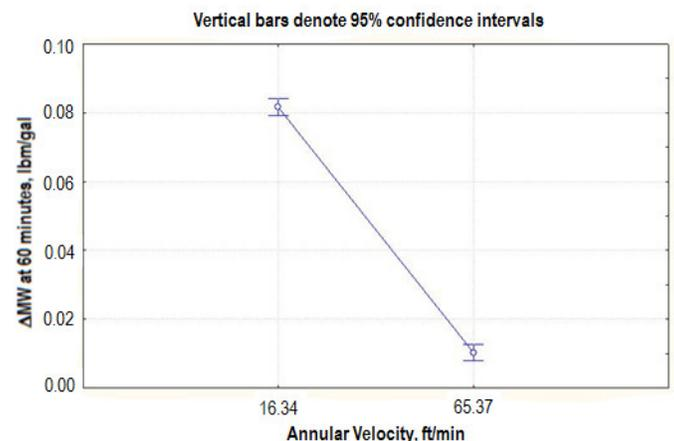
**Figure 3: Overall effect of annular velocity**
