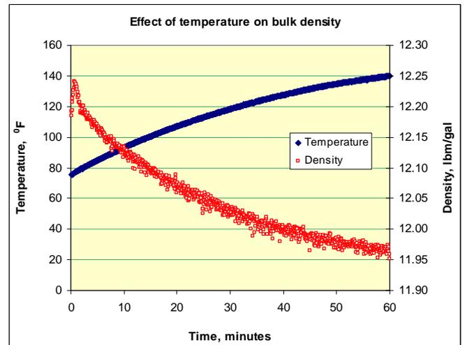
Figure A3: Effect of temperature on bulk density of oil-based drilling fluid
