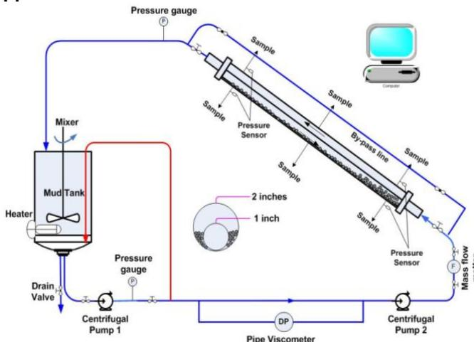
Figure A1: Schematic of the Barite Sag Flow Loop (BSFL)
