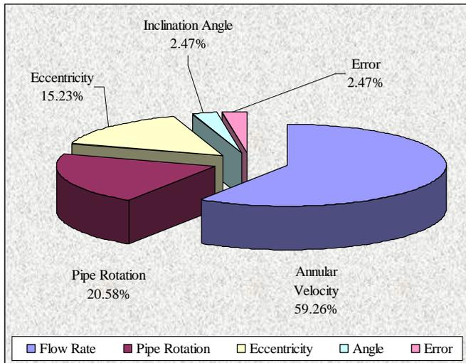
Figure 7: Individual effect of drilling parameters on barite sag
