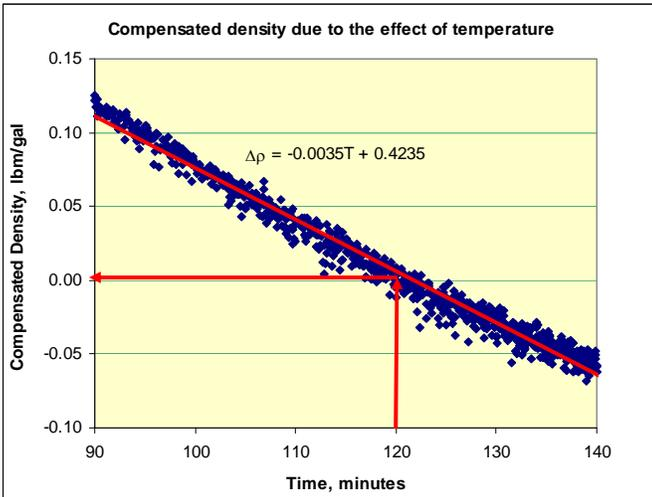
Figure A4: Compensated density due to the temperature effect
