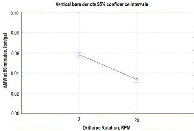
Figure 4: Overall effect of drill-pipe rotation
