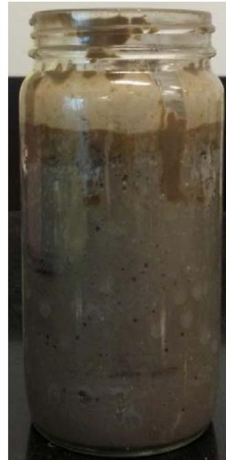
**Figure 2: Fluid sample after long term static aging at 190°F**
