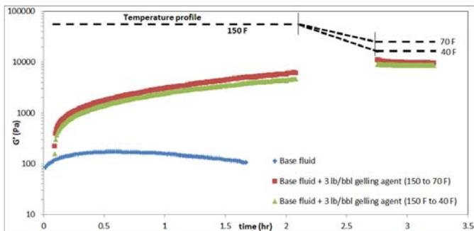
Figure 5: Oscillatory test ( $\omega = 1$  rad/s and  $\gamma = 0.1\%$ ) on parallel plate geometry
