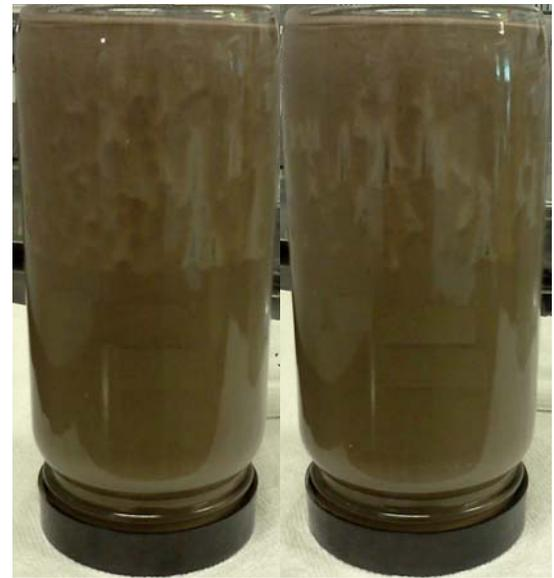
**Figure 3: Fluid with gellant after 7 and 10 hours at 120°F**
