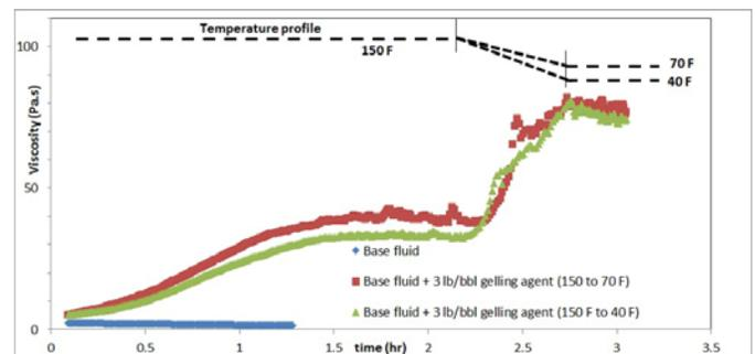
**Figure 4: Rotational test (shear rate = 1.5 s<sup>-1</sup>) on parallel plate geometry**
