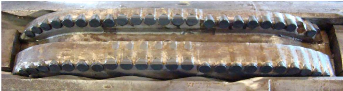
WELL #3, 13-in OD concentric reamer design 2 cutter block in good condition
