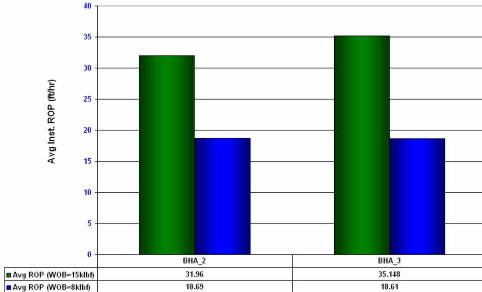
Figure 11 - ROP analysis results for bit #1 and different BHA's and WOB loads
