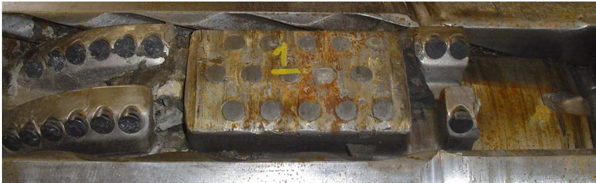
WELL #2, 13-in OD concentric reamer design 1 cutter block with severely damaged lower cutter block (r)
